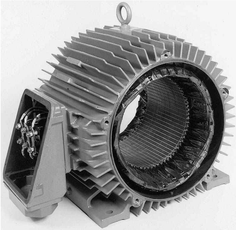
Plate 5.1 Stator of three-phase induction motor. The semi-closed slots of the stator core obscure the active sides of the stator coils, but the ends of the coils are just visible beneath the binding tape. (Photograph by courtesy of Brook Crompton)
