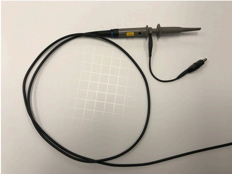
Figure 3.5: Rigol Oscilloscope Probe: http://www.prc68.com/l/RigolDS1052E.shtml
