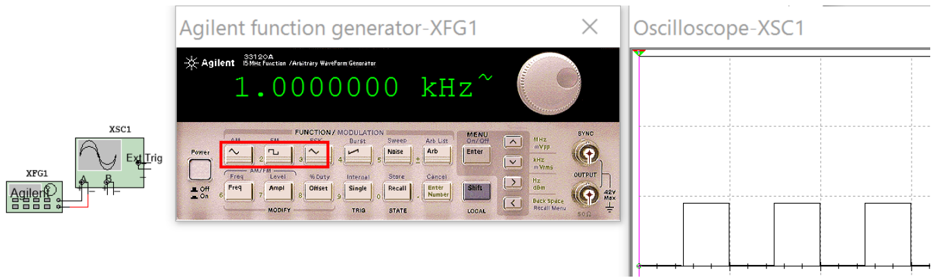
Figure 1.8: Agilent Function Generator and Multisim 2-Channel Oscilloscope.
