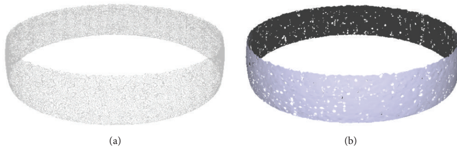
FIGURE 9: (a) Point cloud (79669 points) and (b) surface reconstruction (156135 elementary triangles) of the ceramic calibration sphere.
