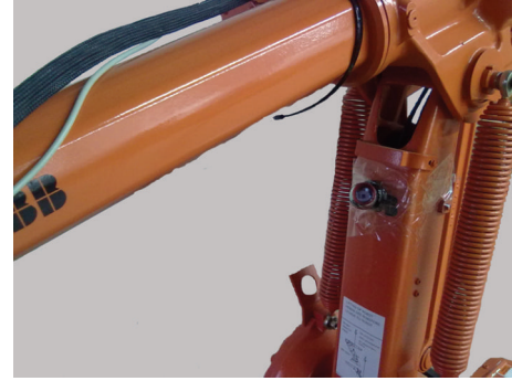
FIGURE 4: The reflector on the axis 2.
