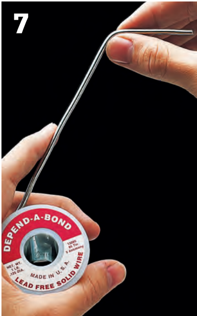
7 Prepare the wire solder by unwinding 8" to 10" of wire from spool. Bend the first 2" of the wire to a 90° angle.
