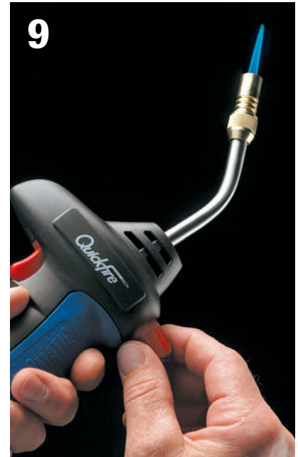
9 Adjust the torch valve until the inner portion of the flame is 1" to 2" long.
