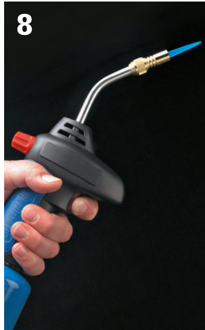
8 Open the gas valve and trigger the spark lighter to ignite the torch.
