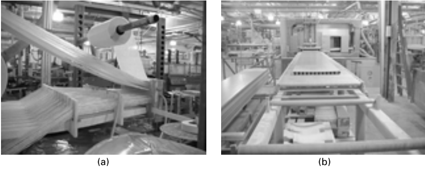
4.1 Pultrusion process (a) fiber guiding and impregnating; (b) forming structural profiles.
