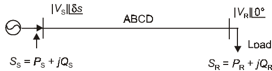
Fig. 6.7: Two bus sample power system.
