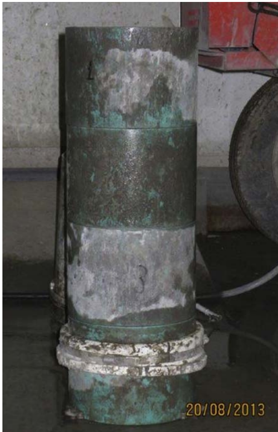
Figure 26.4 Measuring SCC static stability.
