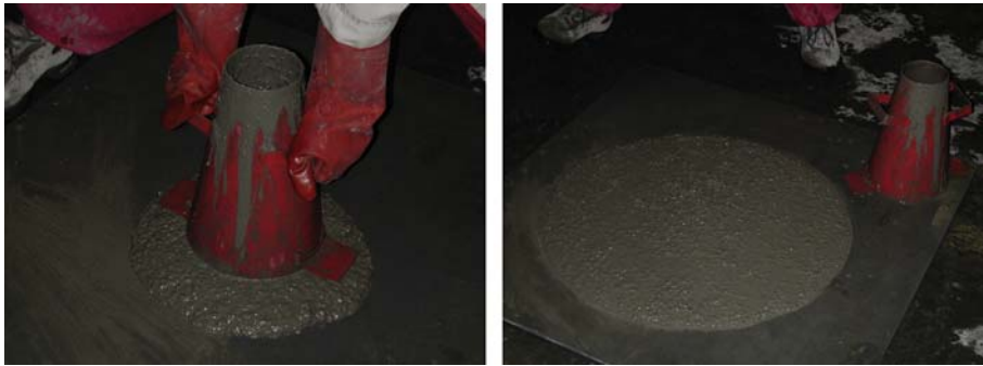
Figure 26.1 Slump flow measurement.
