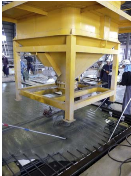
Figure 27.20 The filling of the moulds with UHSC.
