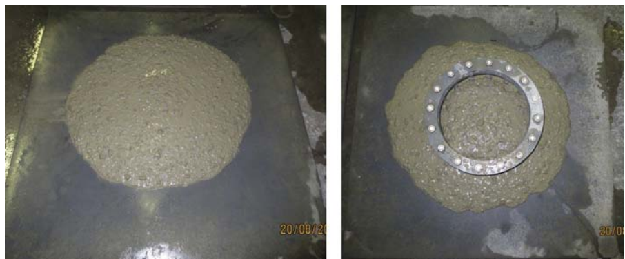
Figure 26.2 Measuring passing ability with a J-ring.
