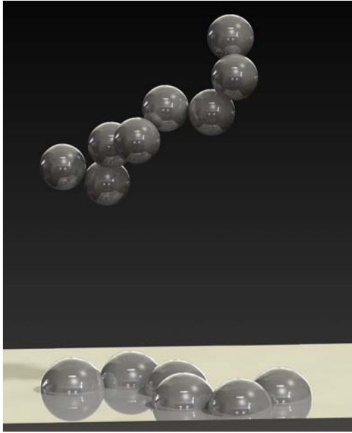
Figure 10.4 Schematic representation of a comb copolymer in solution (chain of spherical cores, each of radius R_C ) and one adsorbed on a mineral surface (chain of hemispheres, each of radius R_C ).
