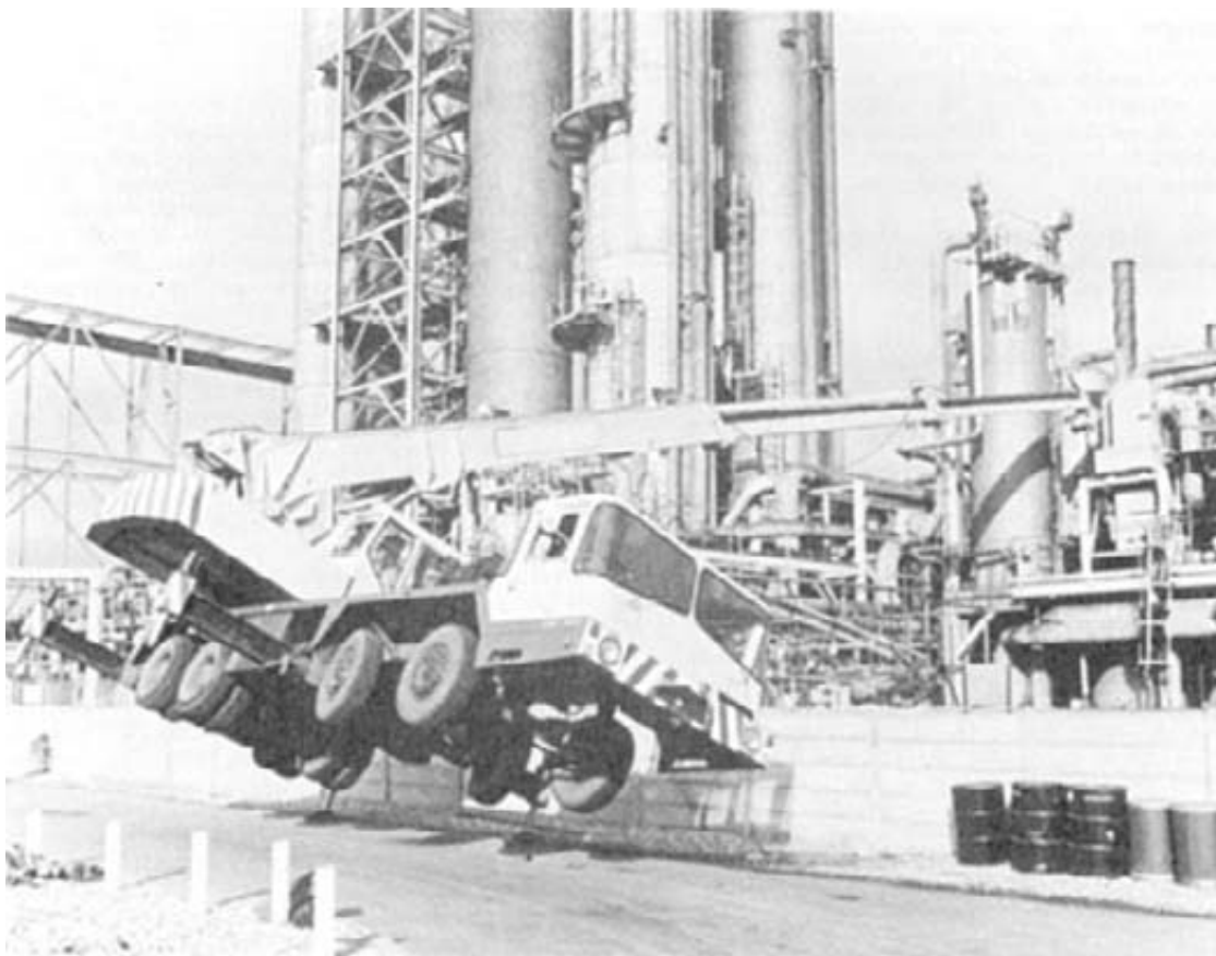
Figure A1.24 Mobile crane overturned on to plant (Anon., 1977n)
