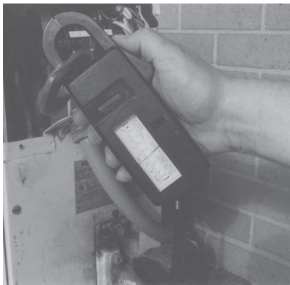
► Figure 3-18 Scale divider used with clamp-on ammeter. The ammeter indicates a value of 3.25 amperes. If the scale divider has a ratio of 10:1, the actual current is 0.325 amps. (Source: Delmar/Cengage Learning)
