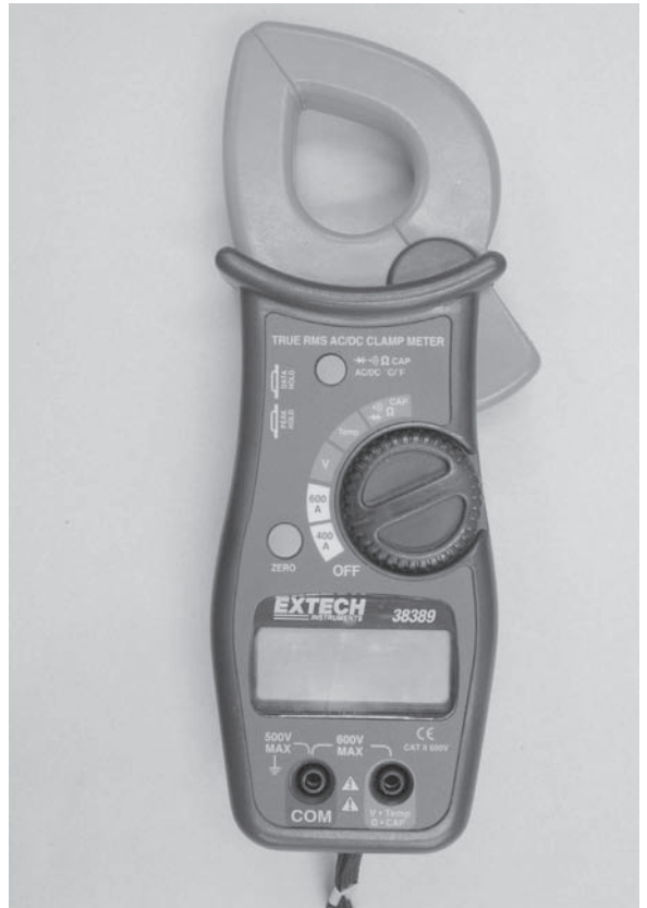
Figure 8-17 Digital meter capable of measuring capacitance. (Source: Delmar/Cengage Learning)
