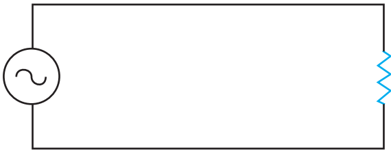
► Figure 7-1 Pure-resistive circuit. (Source: Delmar/Cengage Learning)
