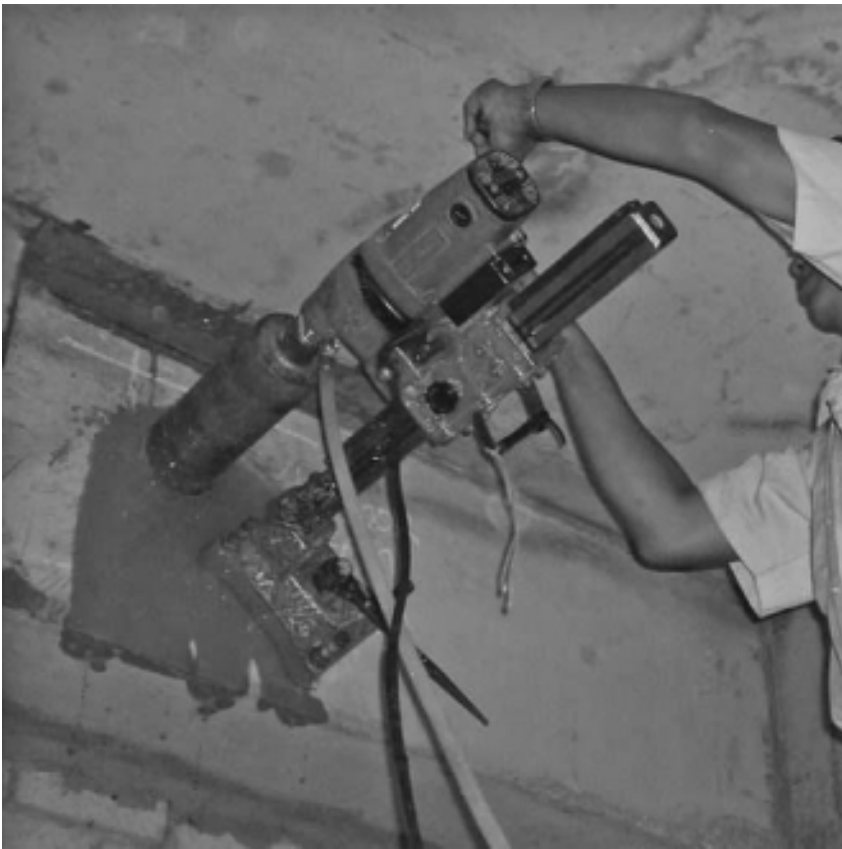
FIGURE 8.3 How to take a core sample.
