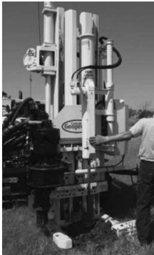
FIGURE 13.4 Rig for the standard penetration test.
