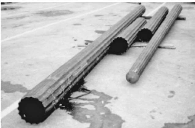
FIGURE 13.13 Raymond shell piles.
