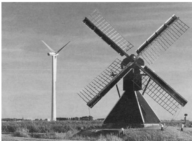
FIGURE 4-5 Old multiblade windmill and modern three-blade wind turbine. (Source: Vestas Wind Systems, Denmark.)
