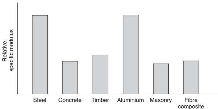
Figure 3.28 Modulus of elasticity per unit weight for structural materials
