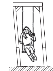
Figure 1.9c Bracing connections fail
