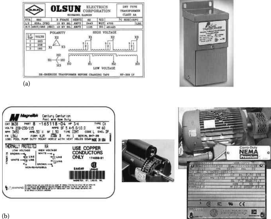
FIGURE 1.10 Sample nameplates: (a) A transformer and (b) an induction machine.
