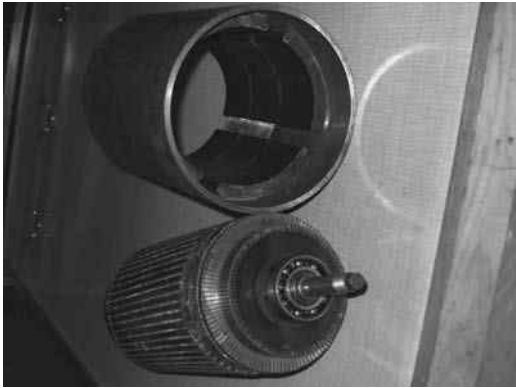
FIGURE 4.1 Typical dc brush–commutator PM motor with its mains parts.
