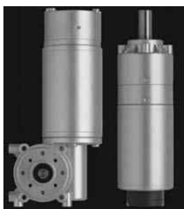
FIGURE 6.4 Automotive electric power steering assist PMSM; and V_{dc} = 12\text{ V} , T_{en} = \text{up to } 1\text{ Nm} , n = 2000\text{ rpm} , n_{max} = 4000\text{ rpm} , and T_{en,max} = 0.3\text{ Nm} with PWM inverter control for variable speeds.
