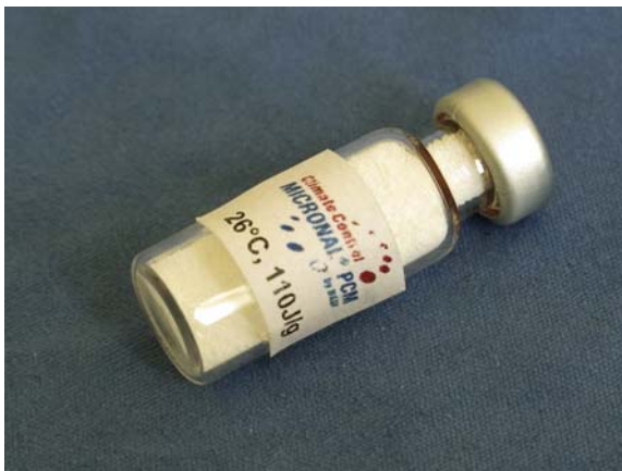
Figure 5.10 BASF Micronal microencapsulated phase-change material. Photo by the author.
