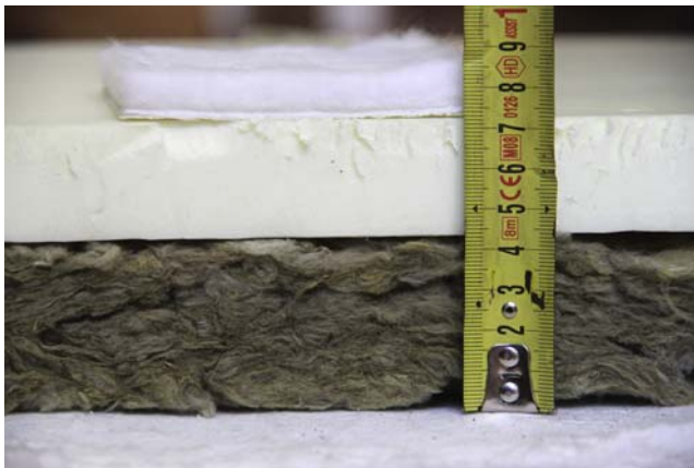
Figure 4.10 Thickness comparison between rock wool, polyurethane, and fiber-reinforced aerogel blanket. Photo by the author.
