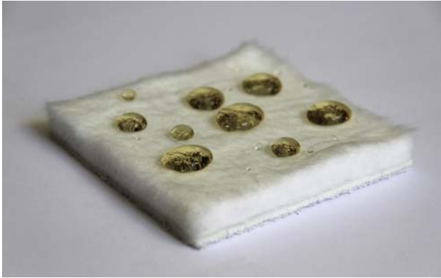
Figure 4.11 Fiber-reinforced aerogel blanket hydrophobic behavior. Photo by the author.
