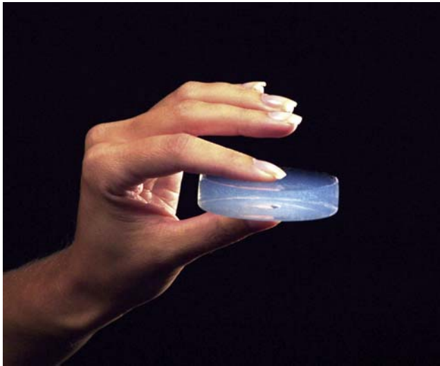
Figure 4.3 Monolithic silica aerogel. Courtesy of Aspen Aerogels Inc.
