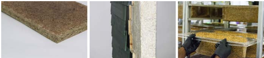
Figure 4.35 Mycelium insulating materials and preparation. Courtesy of Ecovative.
