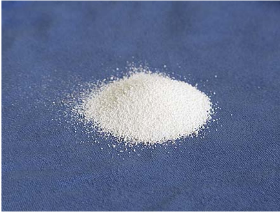
Figure 5.11 BASF Micronal microencapsulated phase-change material. Photo by the author.
