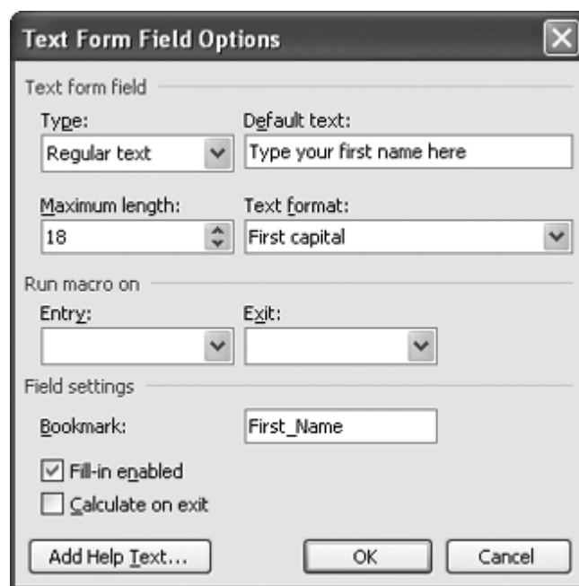
Figure 3-1. Use the Form Field Options dialog box to control whether the form field is enabled (so that the user can fill it in) and to set the name of the bookmark that refers to it. The other options available depend on the type of form field: a text box (as shown here), a checkbox, or a drop-down list.
