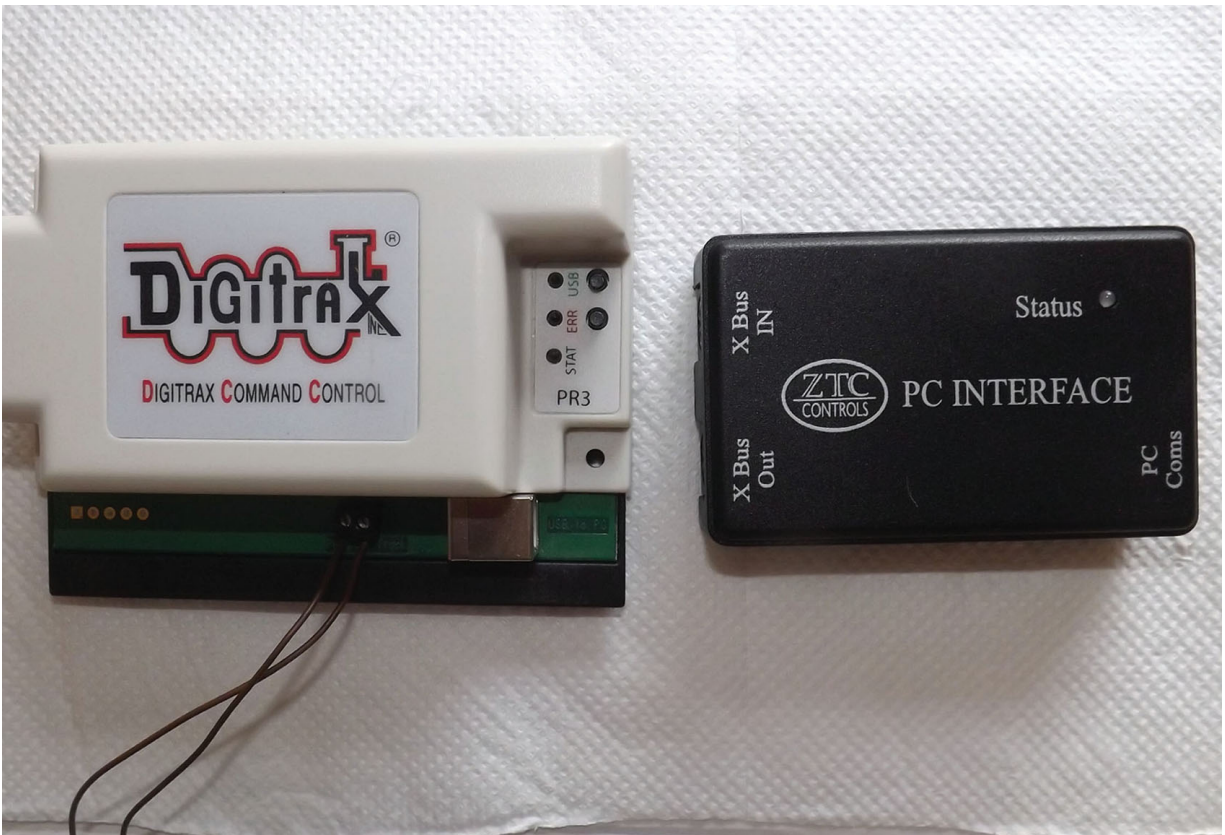
Two computer to DCC interfaces: (left) the American Digitrax; (right) the British ZTC. Unlike the accessory decoders, the interfaces must match the manufacturer's controller.
