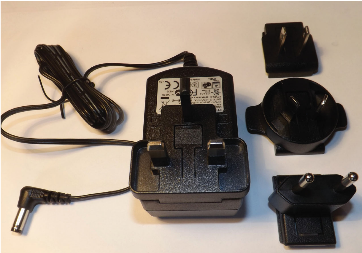
A 12V 1A switch mode power supply. A conventional linear power supply would be much larger in size. On the right are the different adapters for the mains sockets of various countries.
