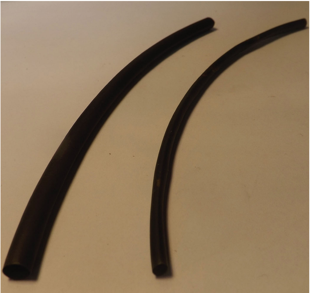
Two different diameters of heat shrink: 4.8mm and 2.4mm. Both will shrink to half their diameter when heated with a hot air gun. Other diameters and colours are readily available.
