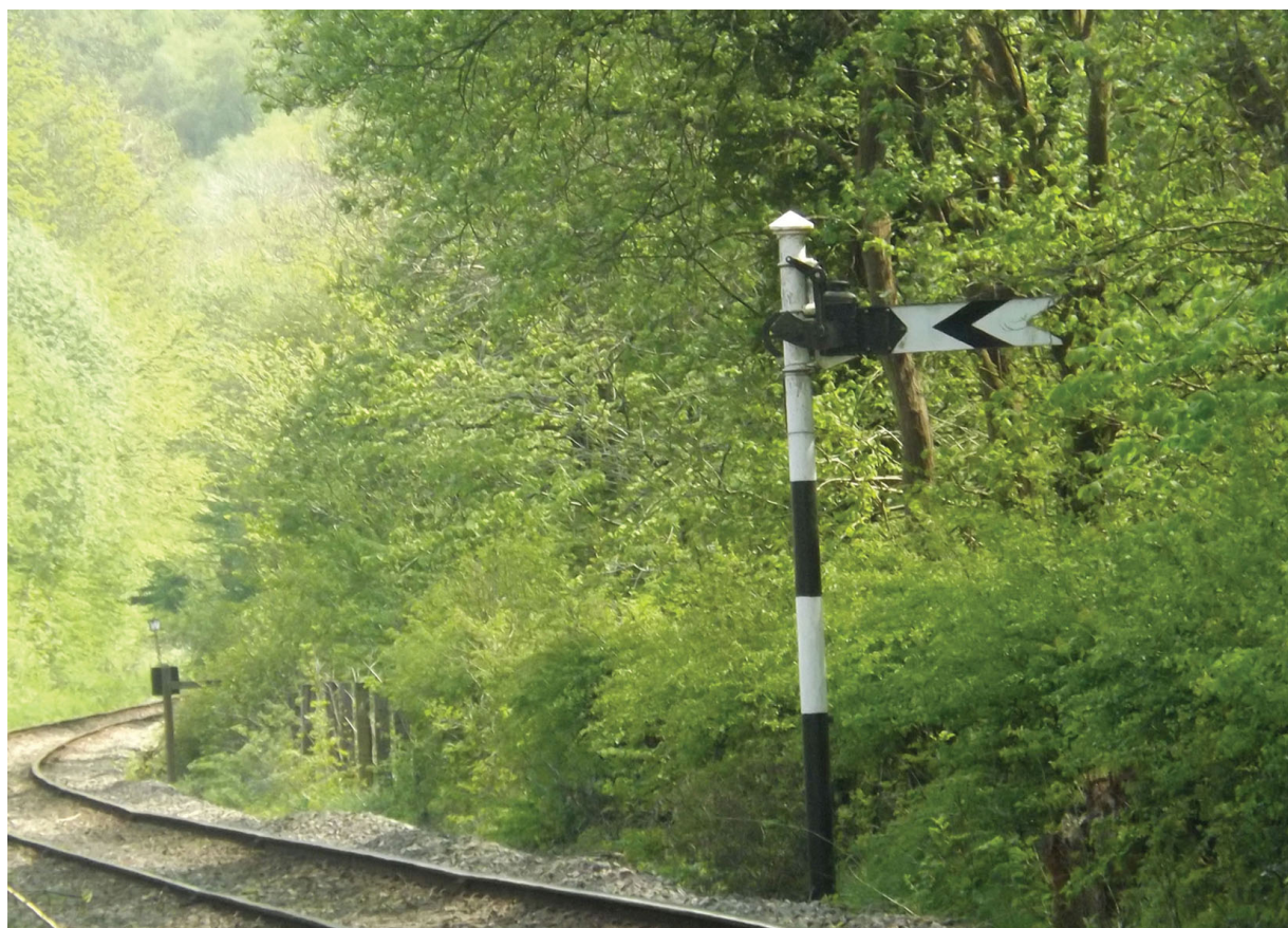
The reverse side of a distant semaphore signal. Note the notch cut out of the arm to identify it as such.
