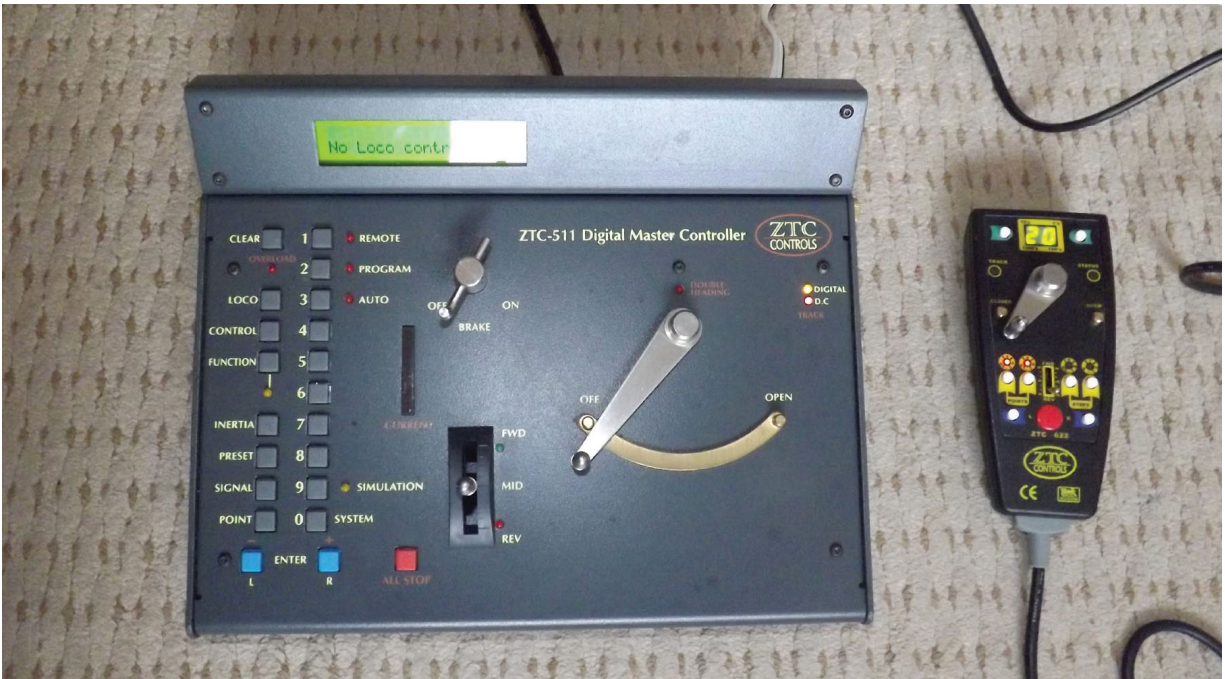
A ZTC DCC controller. As well as controlling the engines it can also be used to control the points. It sends digital signals along the rails to the accessory decoder, which in turn produces the electrical output to the point motor. To the right is a subsidiary hand-held controller for a second operator.
