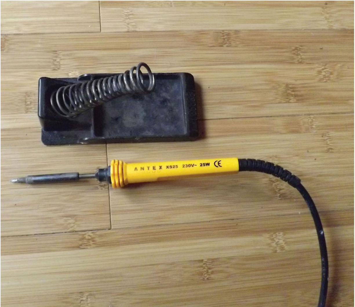
This 25W soldering iron by Antex is designed for lead-free solder and is very suitable for assembling electronic circuits and soldering wires on to switches and tracks. It is a good idea to use a stand when the soldering iron is hot as otherwise it is very easy to have an accident.
