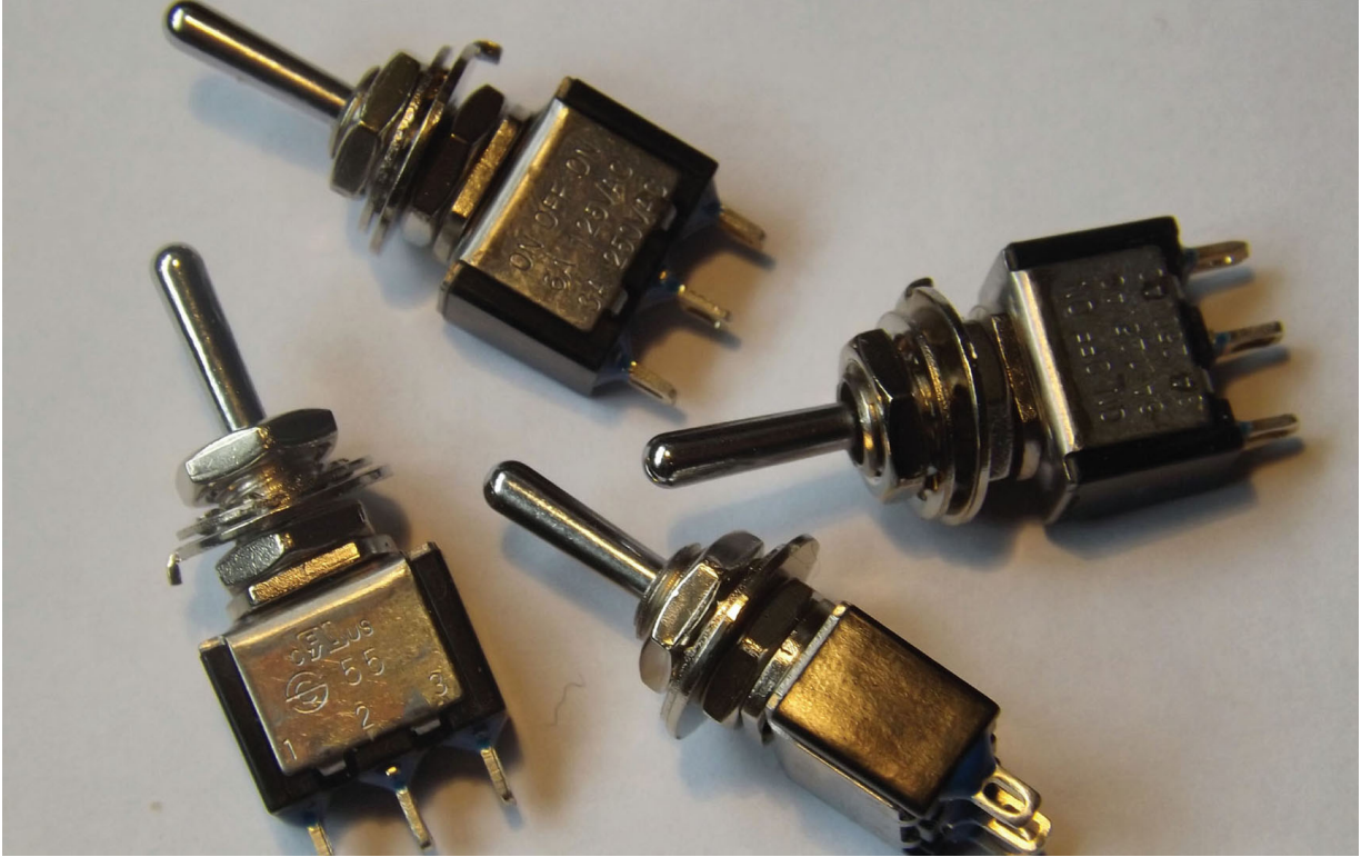
Four toggle switches. The levers are all in the upright position, where no connections are made. Gentle finger pressure pushing them to either side will make a connection.
