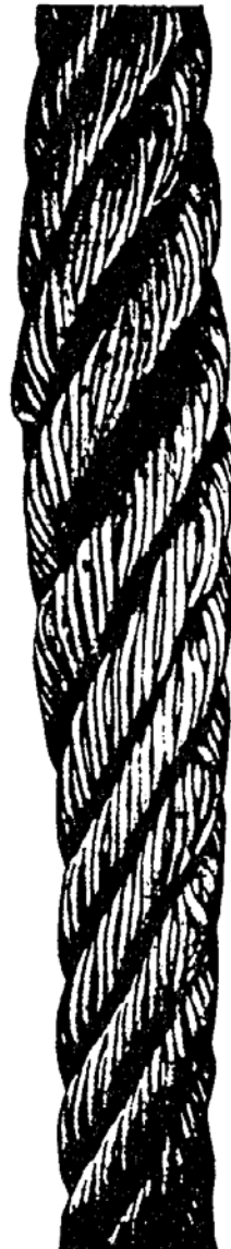
Localized crushing of rope
