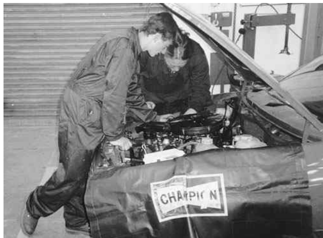
Figure 19.12 A vehicle with protection covers fitted
