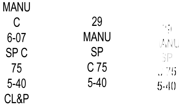
Figure 16.5 Left, brand following the guidelines of ANSI standard 05.1.2008 gives from top to bottom: manufacturer (MANU), which plant the pole (C) came from, month (6) and year of manufacture (07), code for the wood type (SP-Southern Pine), code for the type of preservative (C-creosote), the amount of preservative infused in the pole (.75 lbs per cubic foot), the class (5) and length (40), and the owner (CL&P). Middle, some of this information as contained in pre-WWII and early postwar brands found on the CL&P system. Right, a depiction of the deterioration and lack of full readability typical of pre-WWII brands.
