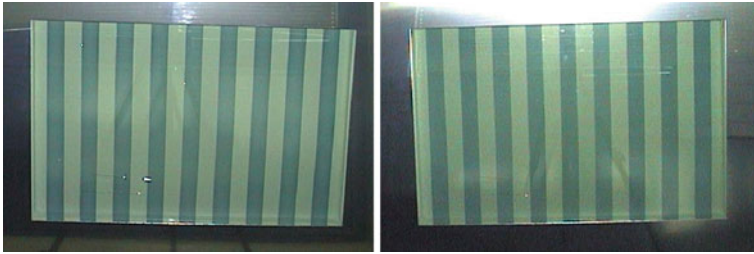
Fig. 12.13 Transparent 50 \times 80 \text{ cm}^2 EC-display (patterned rows) with the configuration glass/FTO/ \text{WO}_3 /nanocomposite electrolyte/ \text{CeO}_2 - \text{TiO}_2 /FTO/glass. Left : after colouration of the rows, Right : after storage the display during 24 h without electrical power supply [109]
