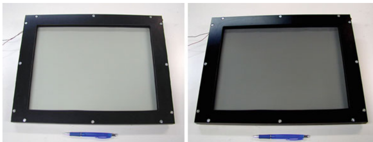
Fig. 12.11 30 × 40 cm 2 prototype of a grey colouring device with the configuration K-glass/Nb 2 O 5 :Mo/nanocomposite electrolyte/(CeO 2 ) x -(TiO 2 ) 1-x /K-glass with a transmission change at 550 nm varying from 60% (bleached state) to 25% (coloured state [38, 131])
