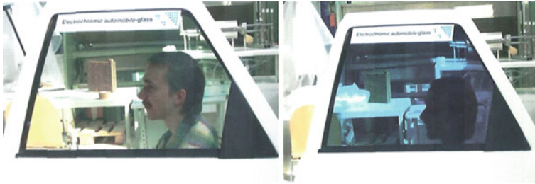
Fig. 12.9 Prototype of a bent EC-window for a car side window. Left: bleached state, right: coloured state, Courtesy from INM
