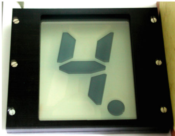
Fig. 12.14 Similar device as in Fig. 12.13 but with patterned pixels. Courtesy from INM
