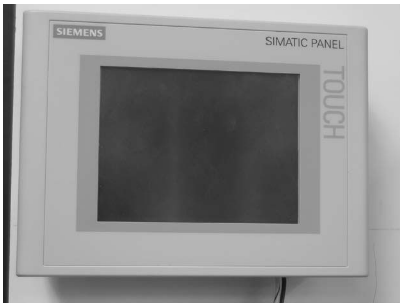
Figure 7-9 Human machine interface (HMI) screen to interact with control systems.
