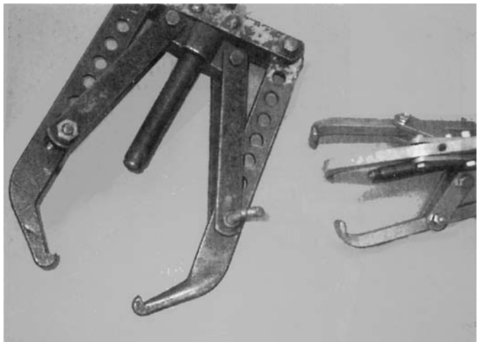
Figure 24-8 Bearing pullers. Use jaws to pull bearing off the shaft.
