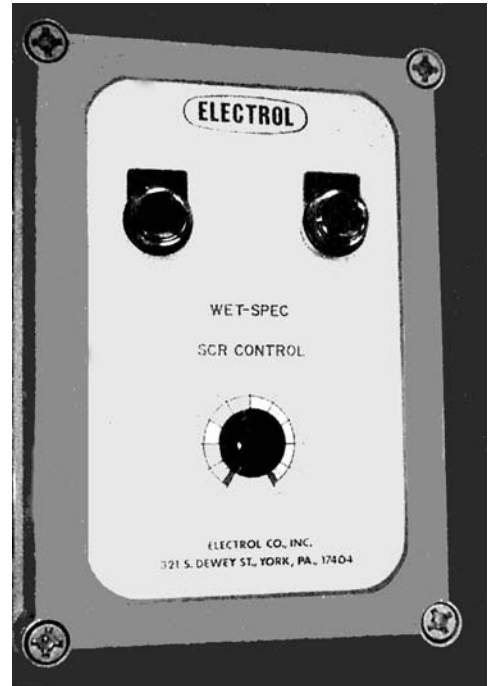
Figure 8-7 Control panel for SCR-controlled DC motor drive.
