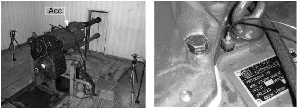
Figure 5.24 Back-to-back test rig at the TATRA Company a.s. and the accelerometer location.
