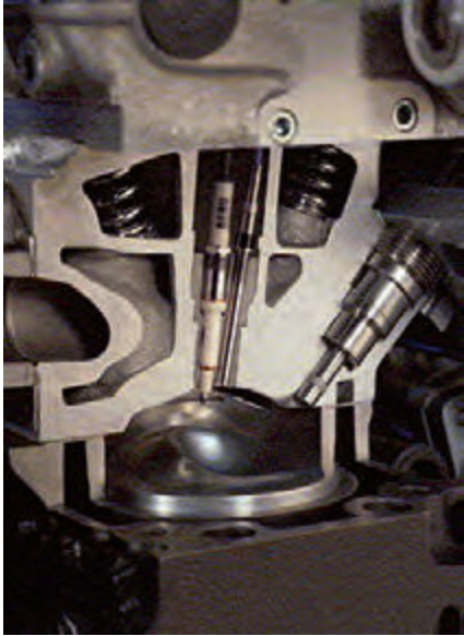
Figure 5.23 Cylinder pressure sensor mounted in the engine
