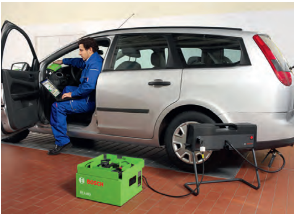
Figure 3.21 Exhaust gas measuring system in use (Source: Bosch Media)
