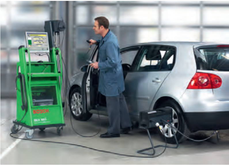
Figure 6.18 Exhaust gas analyser
