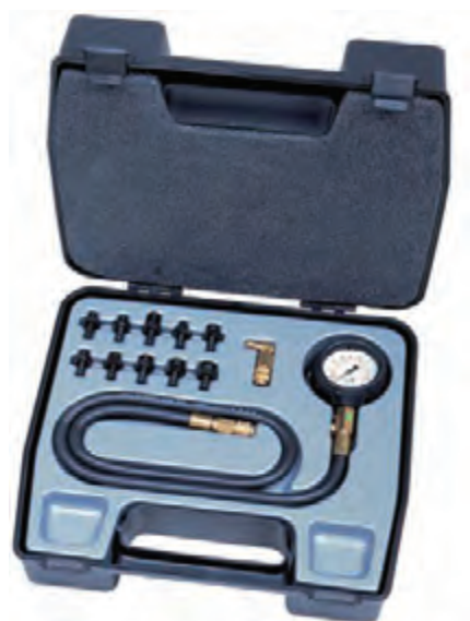
Figure 6.75 Oil pressure testing kit
