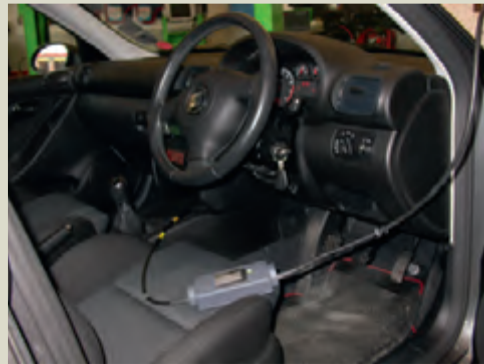
Figure 3.12 Connect the serial lead to the diagnostic socket
