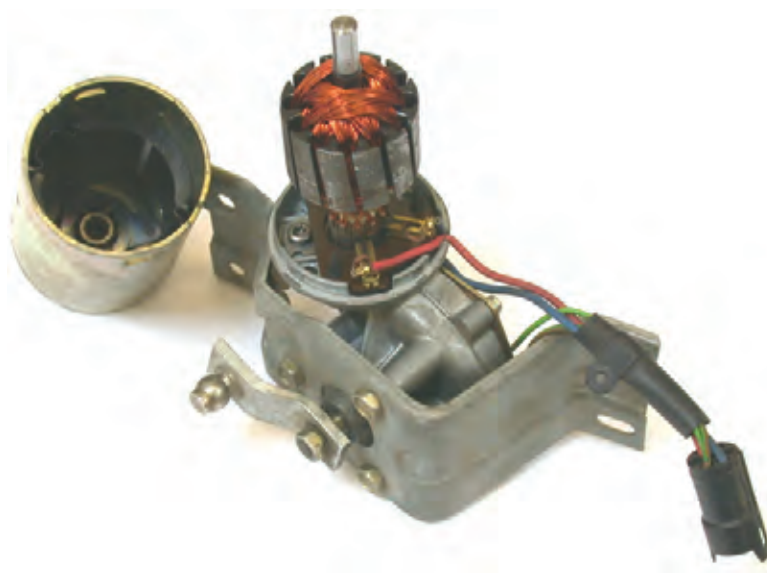
Figure 8.34 Wiper motor using three brushes for two-speed operation
