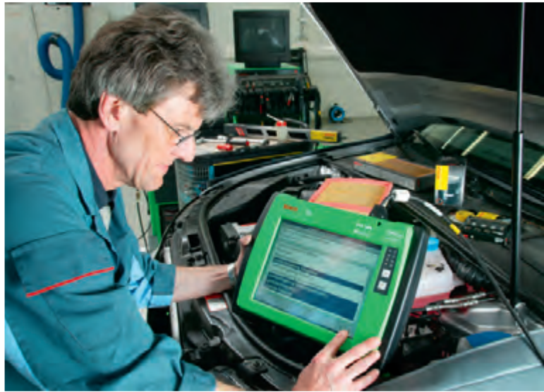
Figure 3.10 Diagnostic system in use (Source: Bosch Media)
