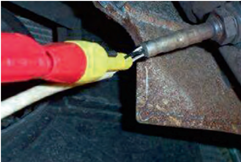
Figure 4.23 Titania knock sensor in position
