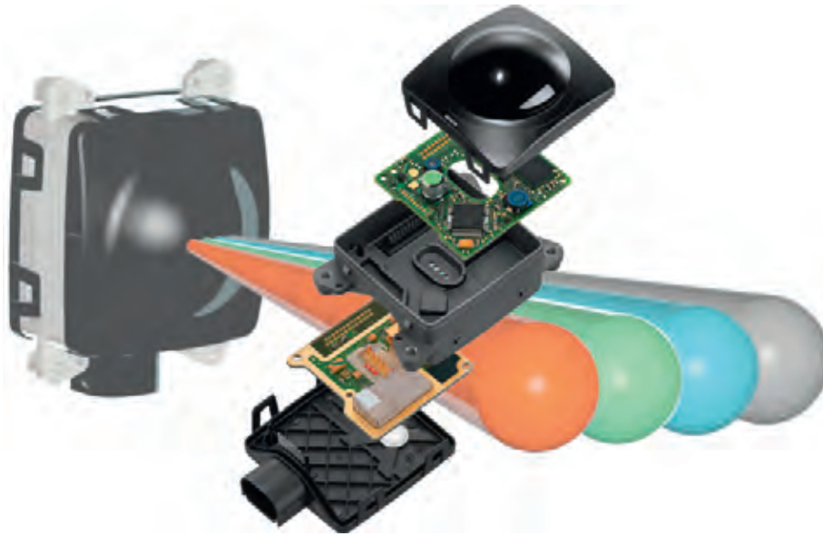
Figure 8.82 Headway sensor and control electronics
