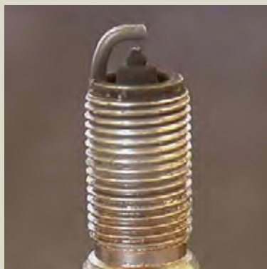
Figure 6.35 Carbon fouled (platinum plug)
