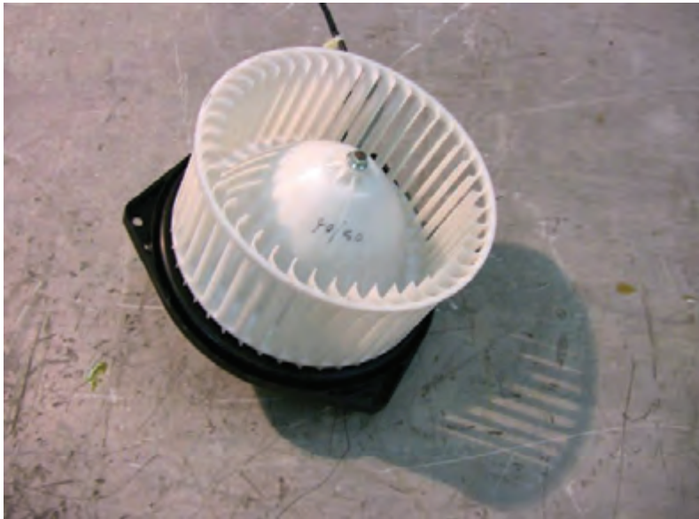
Figure 8.73 Blower motor and fan
