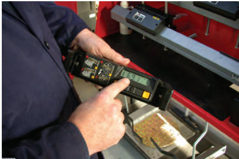
Figure 7.26 Laser alignment systems give digital readouts
