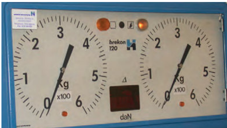
Figure 7.6 Gauges on a rolling road brake tester
