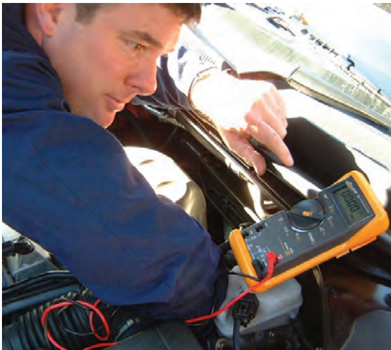
Figure 8.78 Circuit voltage testing
