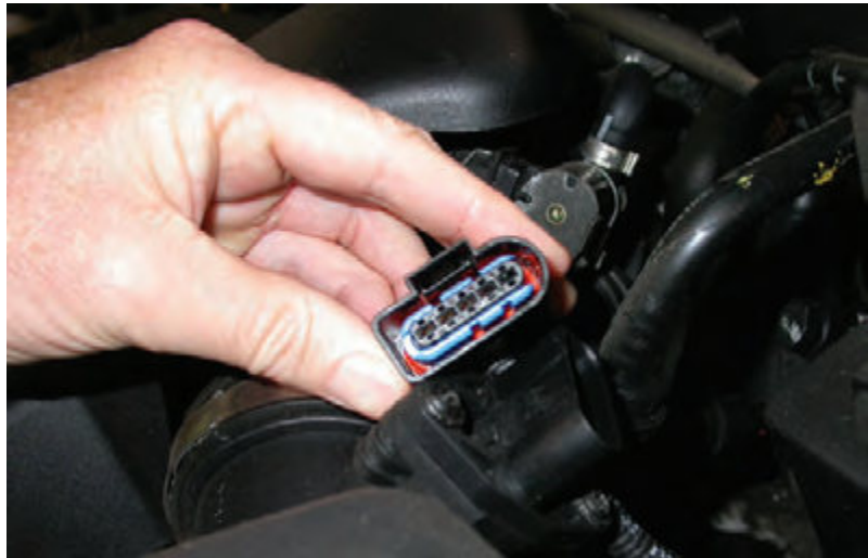
Figure 6.65 Airflow meter under test
