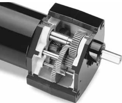
Combination of spur and helical gears can be seen in this cutaway view of a sub-fractional horsepower parallel-shaft gearbox. Note multiple gear stages.
