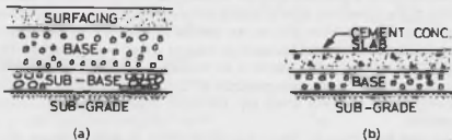
Fig. 29.1 (a) Flexible Pavement.
