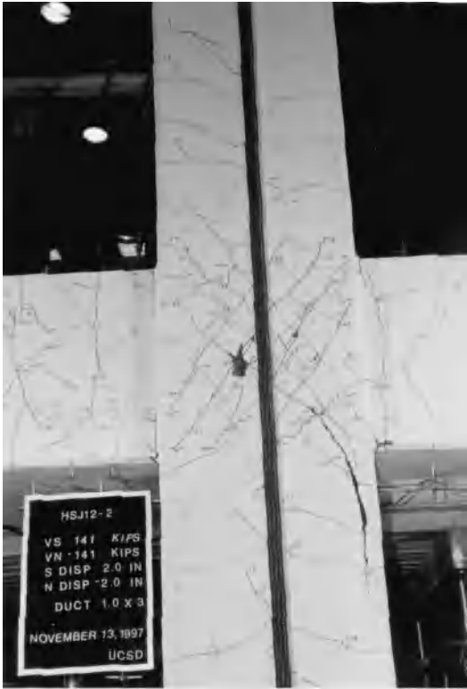
Figure 2.3.2 Joint shear cracks are widening and extending. The cover has begun to spall.
