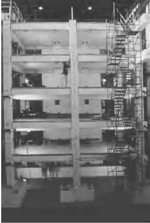
Photo 3.1 Hybrid precast wall panel test program, PRESSS Program. (Courtesy of Englekirk Partners, Inc.)
