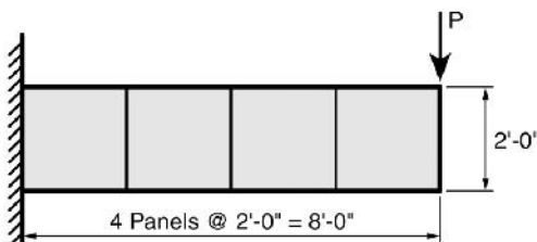
Figure 1.3.11 Beam shear deflection model.
