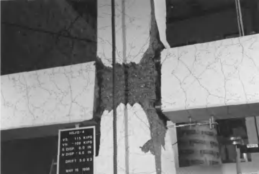
Figure 2.3.21 HSIJ2-#4 third full cycle of 6.0-in. displacements.
