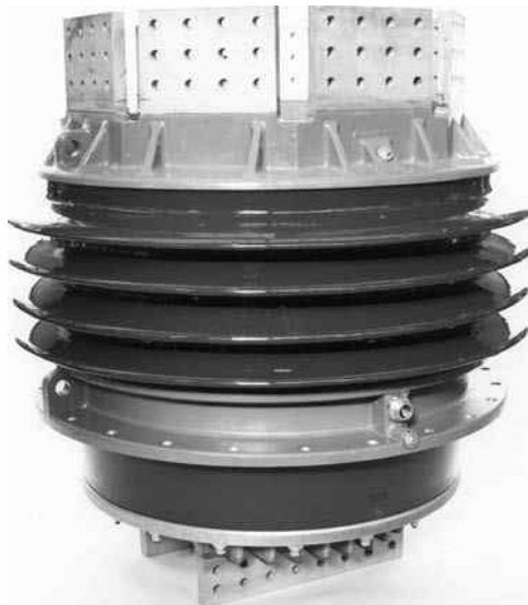
Figure 12.12 36 kV 31,500 A resin-impregnated paper transformer/air bushing
