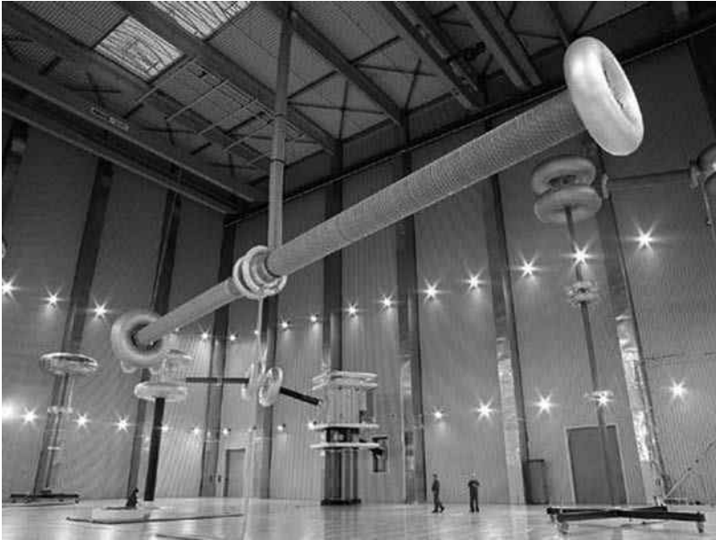
Figure 12.19 Bushing tests at HSP Laboratory, Cologne
