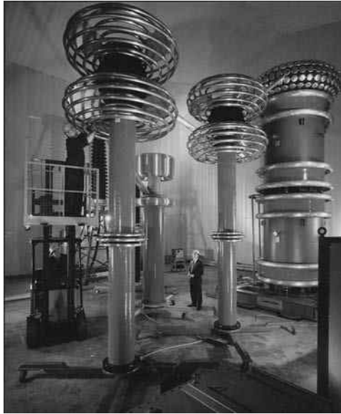
Figure 6.16 Resonant test system for 650 kV, 31 A AC
