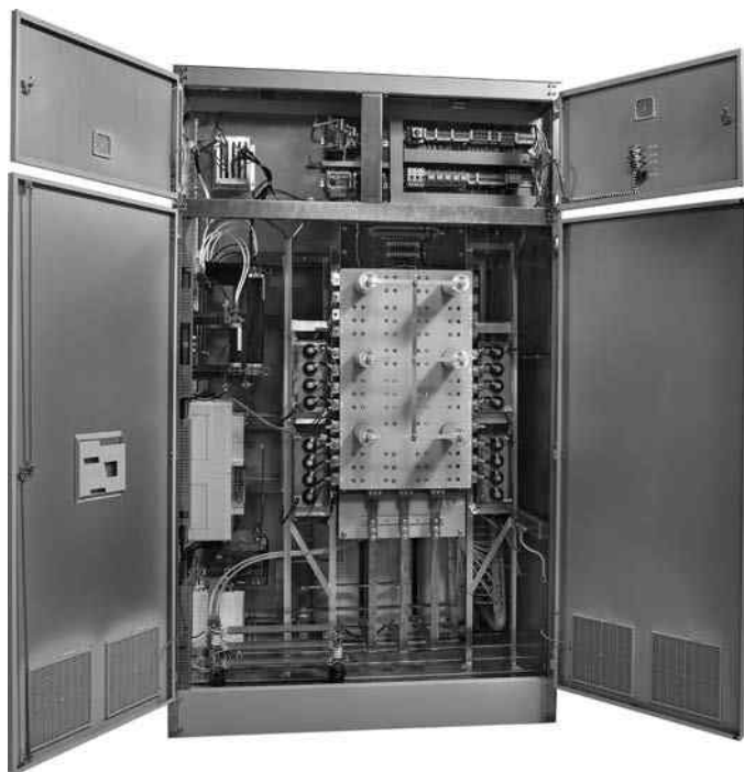
Figure 4.26 Picture of 2 kV 2 MVA cubicle-based STATCOM
