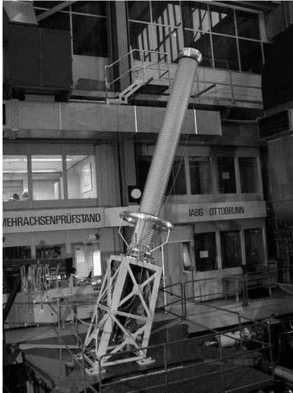
Figure 12.20 Seismic withstand test on polymer transformer bushing
