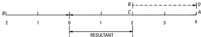
Figure 1-24 Diagram used to determine the resultant of two directly opposed forces.
