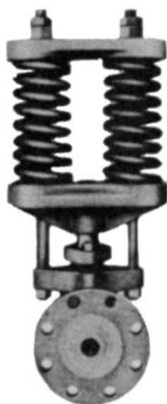
Figure 7-15 A shock-absorbing alleviator. Hydraulic system shocks are absorbed safely and smoothly by means of a packed spring-loaded plunger that rises to relieve sudden pressure surges.
