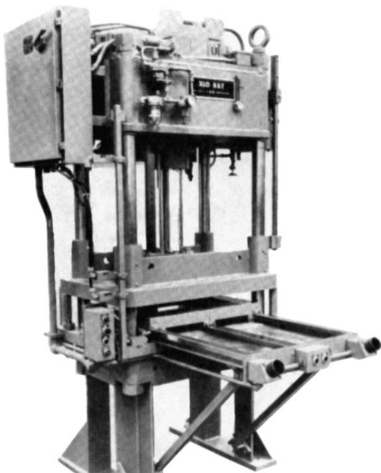
Figure 9-3 A 28-ton hydraulic trim press.
