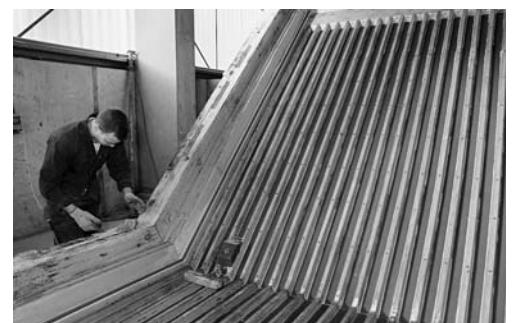
Mould with timber patterning
