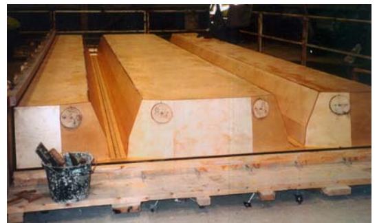
Precast beam mould
