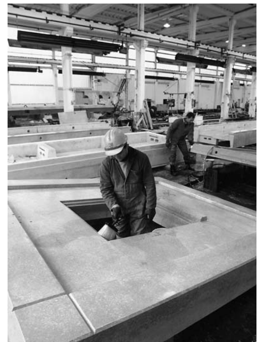
Cleaning edges of precast panel before despatch
