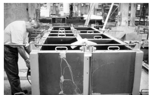
Moulds for precast blocks
