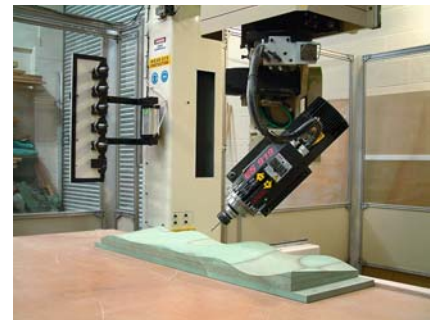
Top and middle: Robotic router machine Bottom: Latex being poured into MDF mould
