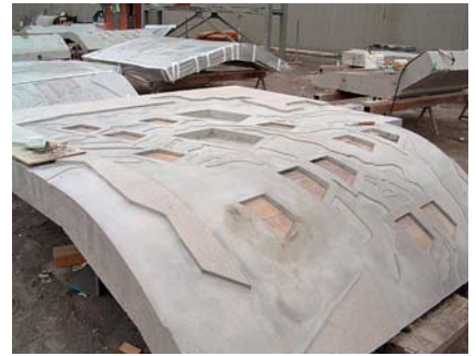
Precast panel before finishing
