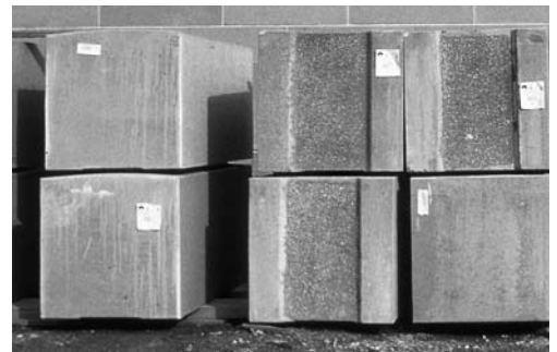
Special stone blocks with location reference
