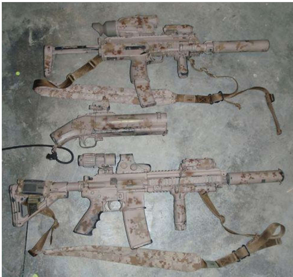
My primary weapons: a Heckler & Koch MP7 with suppressor (top); a highly modified M79 40mm grenade launcher, a.k.a. the “pirate gun” (middle); and a Heckler & Koch 416 assault rifle with a ten-inch barrel and suppressor (bottom).
