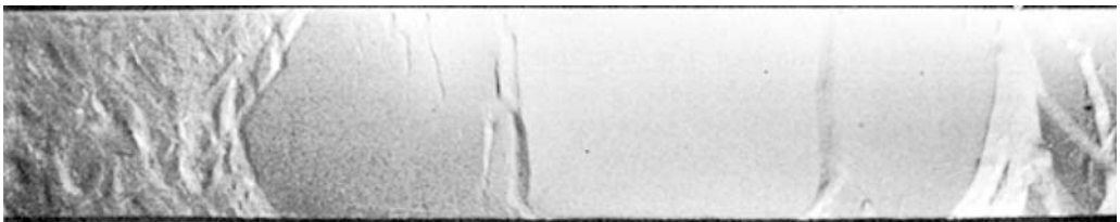
Figure 12.18. Lüder's bands on a low carbon steel tensile specimen. From S. Kalpakjian, Mechanical Processing of Materials , Van Nostrand, 1967, p. 194. Courtesy of J. F. Butler, Jones and Laughlin Steel Corp.
