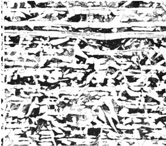
Figure 13.12. Microstructure of a steel plate consisting of bands of pearlite (dark regions) and ferrite (light regions). From Metals Handbook , Vol. 7, eighth ed., ASM, 1972.
