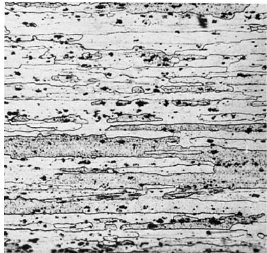
Figure 13.11. Directional features in the microstructure of a 2024-T6 aluminum sheet include grain boundaries and aligned and elongated inclusions. From Metals Handbook , Vol. 7, eighth ed., ASM, 1972.
