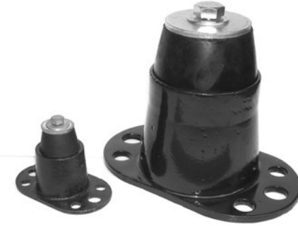
Figure 5-3 Seismically rated elastomeric mounts. The mount on the left (75 mm tall) has a nominal load rating of about 40 kg. The mount on the right (165 mm tall) has a nominal load rating of as much as 700 kg.
