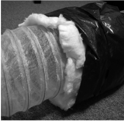
Figure 2-37 Flexible duct with spunbond nylon inner liner.
