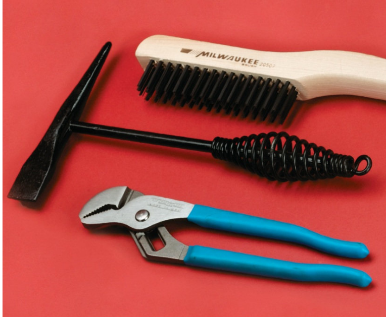
Useful tools for shielded metal arc welding are a pliers, chipping hammer, and wire brush.
