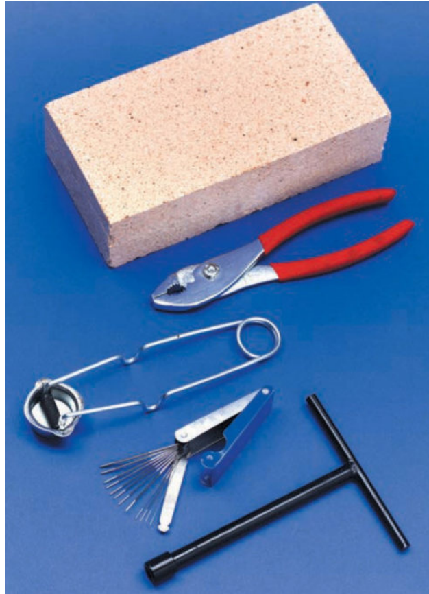
Tools for oxyacetylene welding include fire bricks, pliers, striker, tip cleaner, and acetylene tank wrench.
