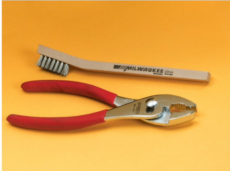
Pliers and a stainless steel wire brush are handy for gas tungsten arc welding.
