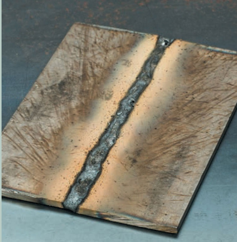
Flux cored wire welds are covered with a layer of slag.
