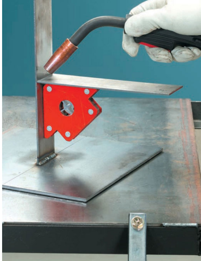
A right angle magnetic clamp makes welding the branches an easy task.
