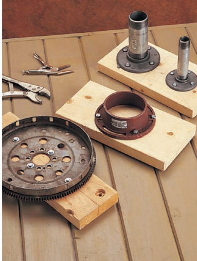
Bending jigs can be made from any rigid circular item. An engine fly-wheel, toilet flange, and various pipe sizes are shown here.
