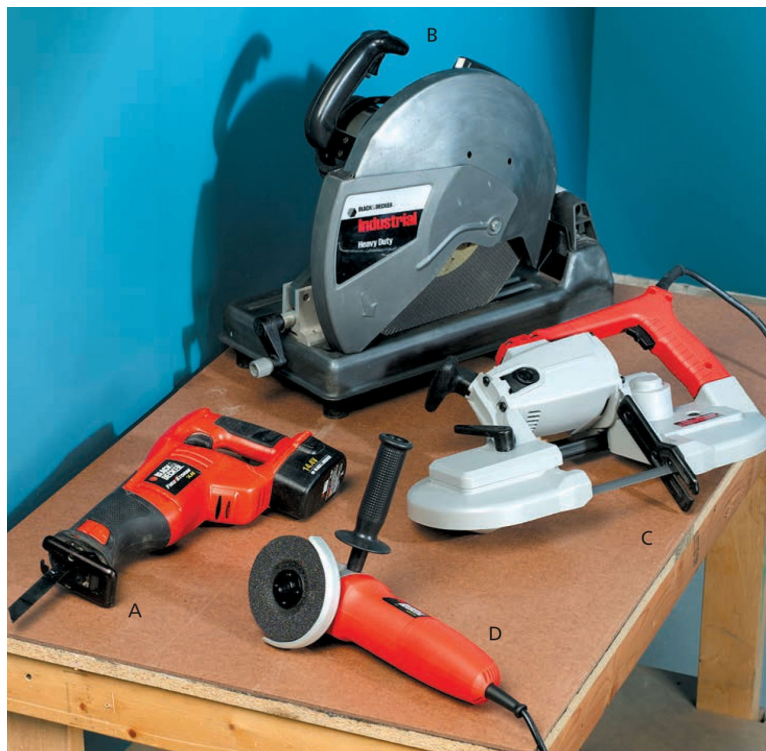
Power tools for a welding shop (above photo) include: A. reciprocating saw, B. chop saw, C. portable band saw, D. angle grinder.
