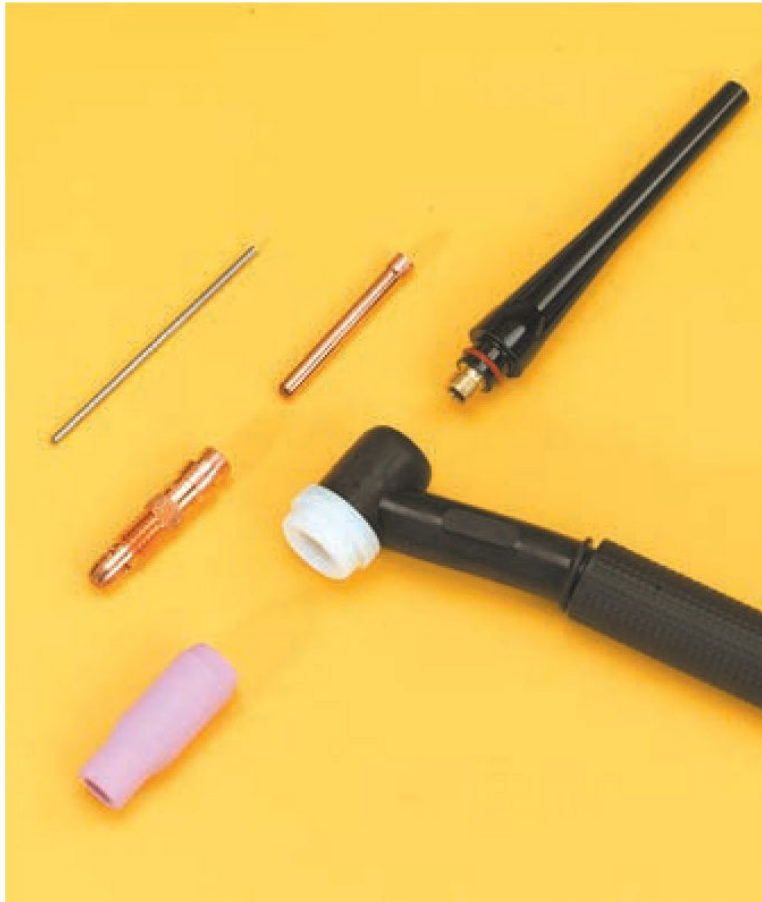
A gas tungsten arc welding torch includes the electrode, collet body, collet, cup, backcap, and torch body with heat shield.
