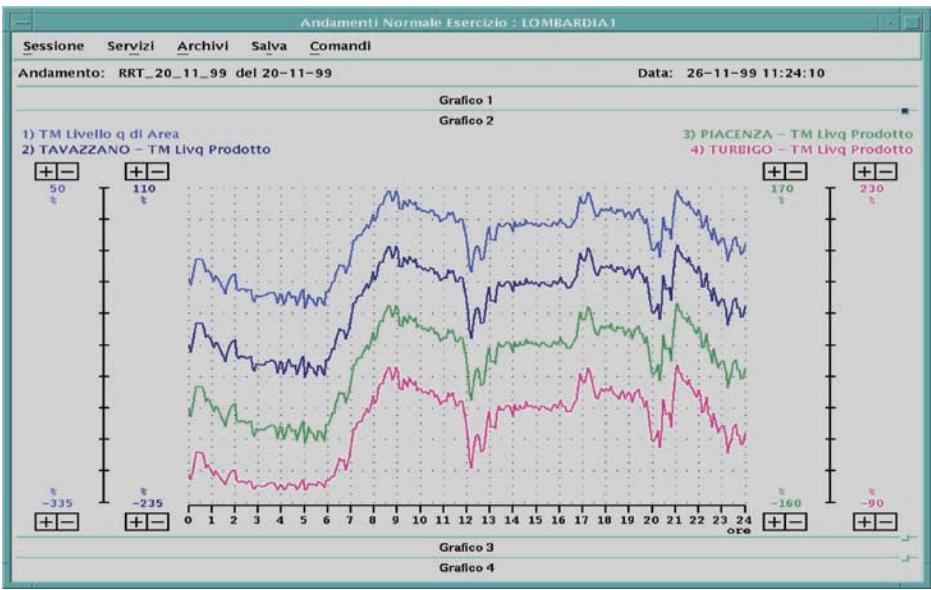
Figure 7.80. Daily reactive power profiles of Piacenza, Turbigo, and Tavazzano control power stations under the remote control of the Milan RVR to regulate the Baggio pilot node as in Figure 7.79.
