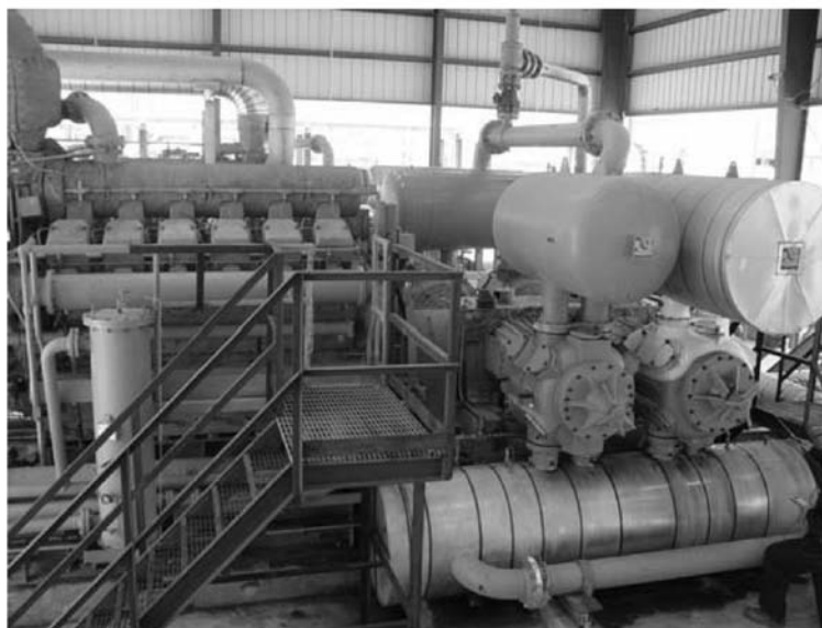
Figure 13-26. 2000 hp (1491 kW), 900 rpm, gas engine driven 3-stage propane refrigeration compressor.
