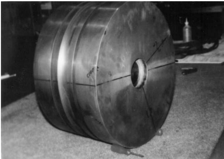
Figure 11-8, Compressor Piston on Inspection Table.
