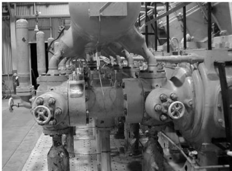
Figure 13-15. Original problematic valve-in-head cylinders required disturbing the outboard piping connections to access the piston, piston rod and packing.
