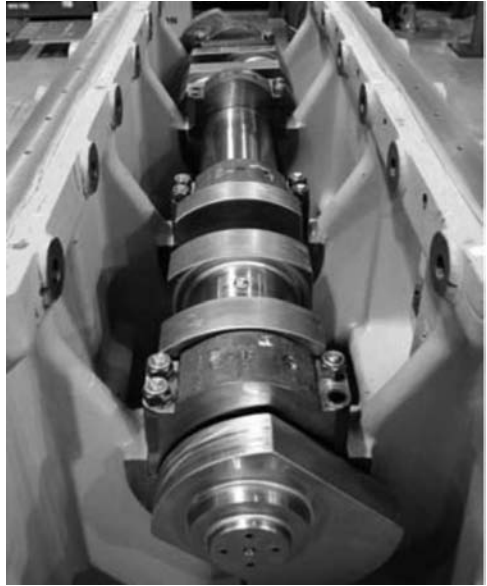
Figure 3-17. Superior MH/HW Compressor Crankshaft Made From Either Forged Or Billet Heat Treated SAE 4140 Steel Courtesy of Cooper Cameron Corporation.
