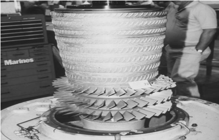
Figure 11-3. Axial Compressor Rotor Surge Damage
