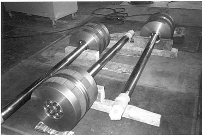
Figure 3-22. Three Piece Cast Iron Pistons With TFE Riders And Flanged Rods Courtesy of ACI Services, Inc.
