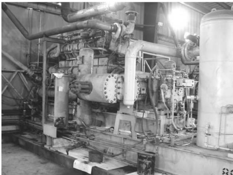
Figure 13-27. Obsolete KOCA-2 compressor prior to conversion.
