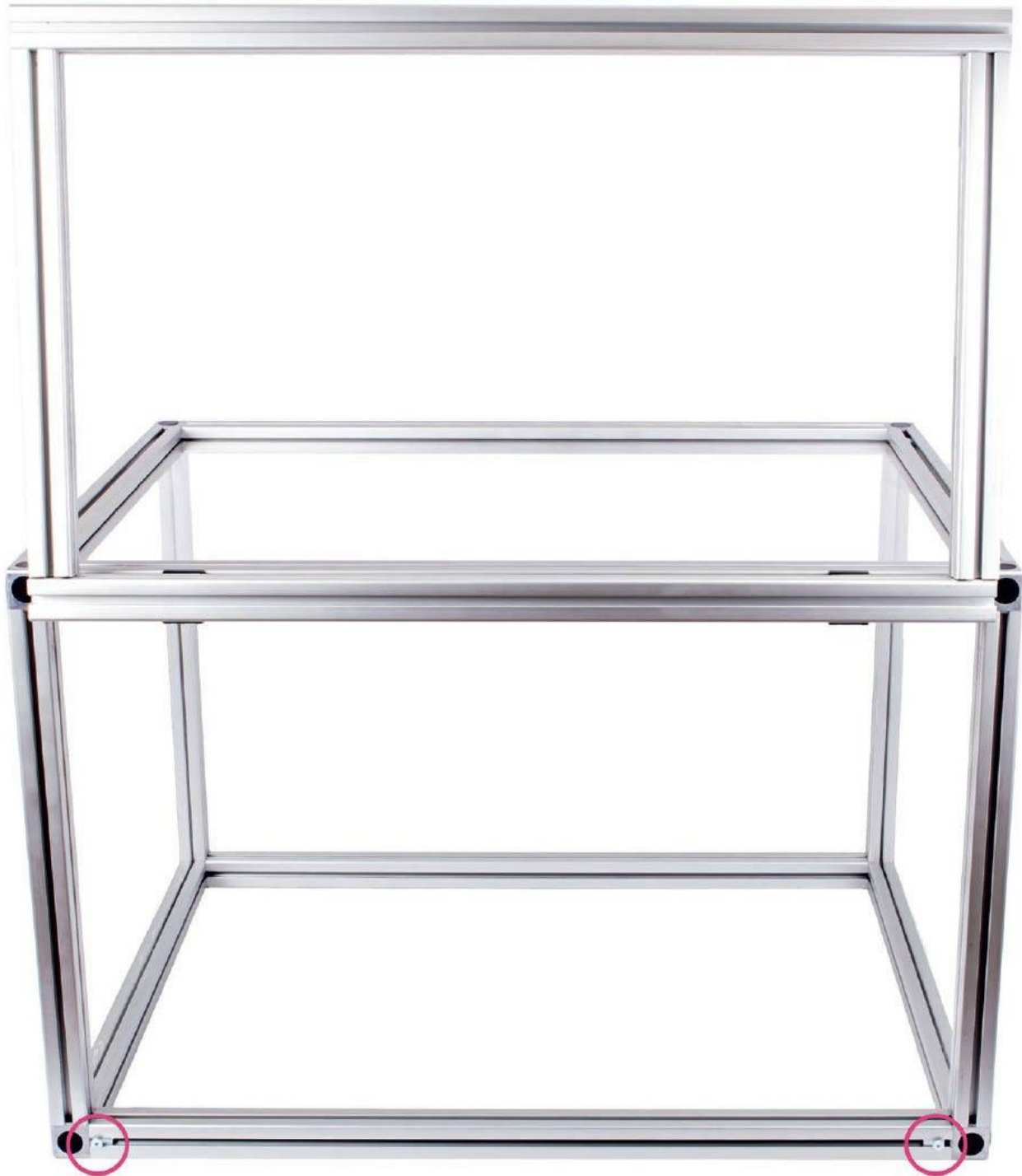
Fig. 5.3 The finished enclosure with the front flap open and the additional T-slot nuts marked in red
