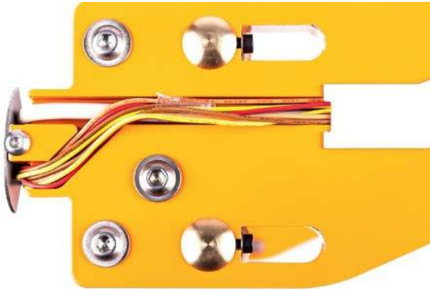
Fig. 2.54 Laying and threading the cables
