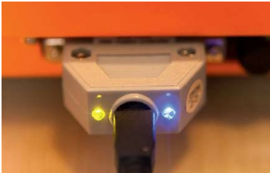
Fig. 7.6 These LEDs show that the UC100 is ready for operation
