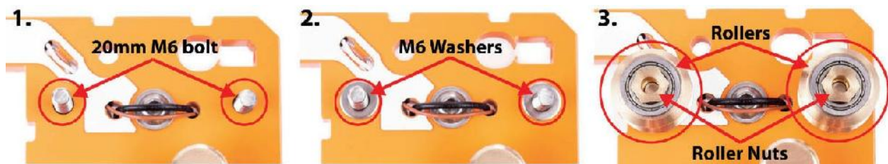
Fig. 2.15 Mounting the remaining rollers on the front of the X-Z connector
