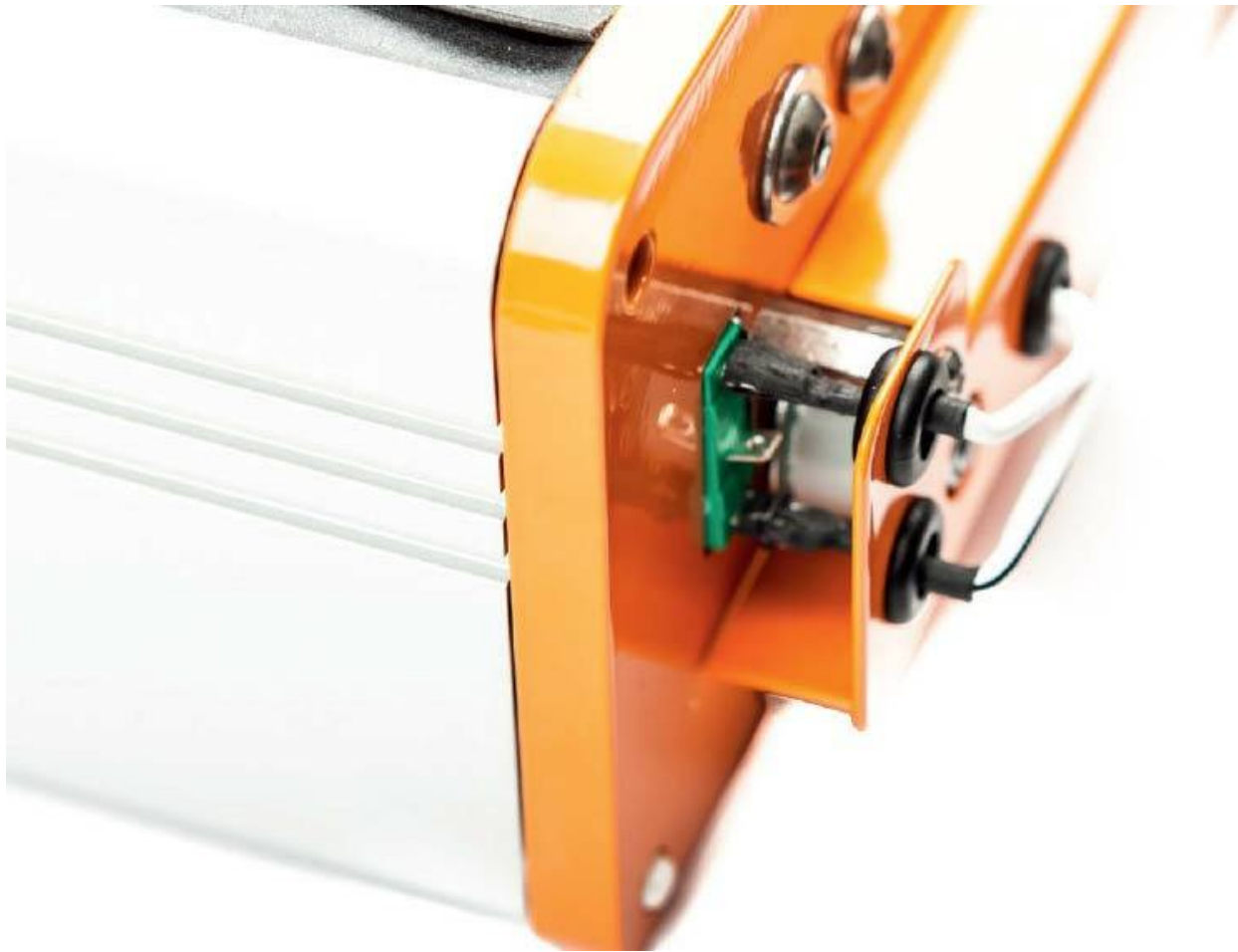
Fig. 2.82 Connecting and laying the end switch cable
