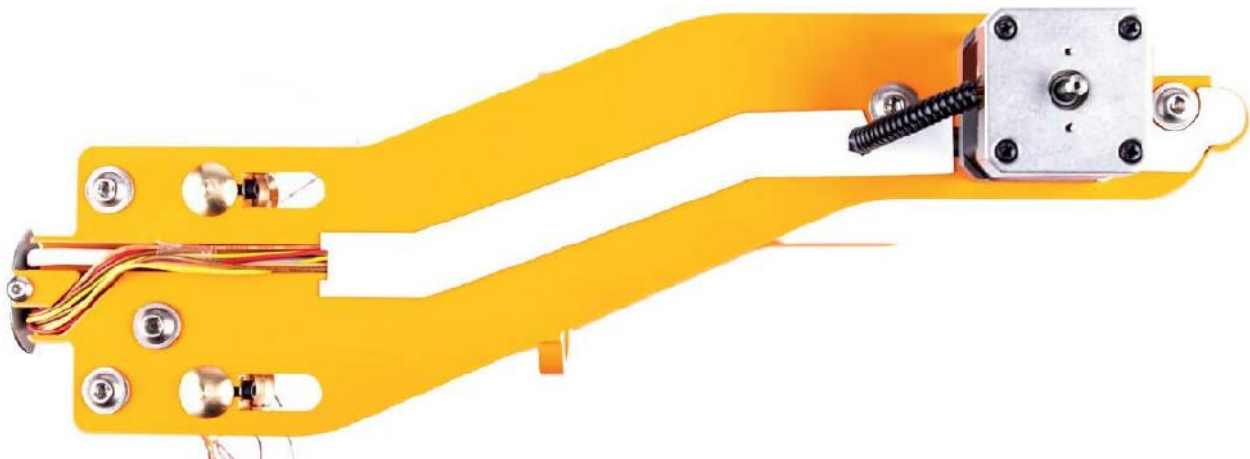
Fig. 2.53 The stowed and covered motor cables
