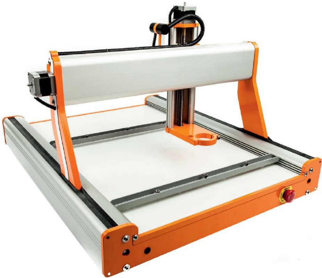
Fig. 1.2 A hobby-grade 3-axis gantry milling machine
