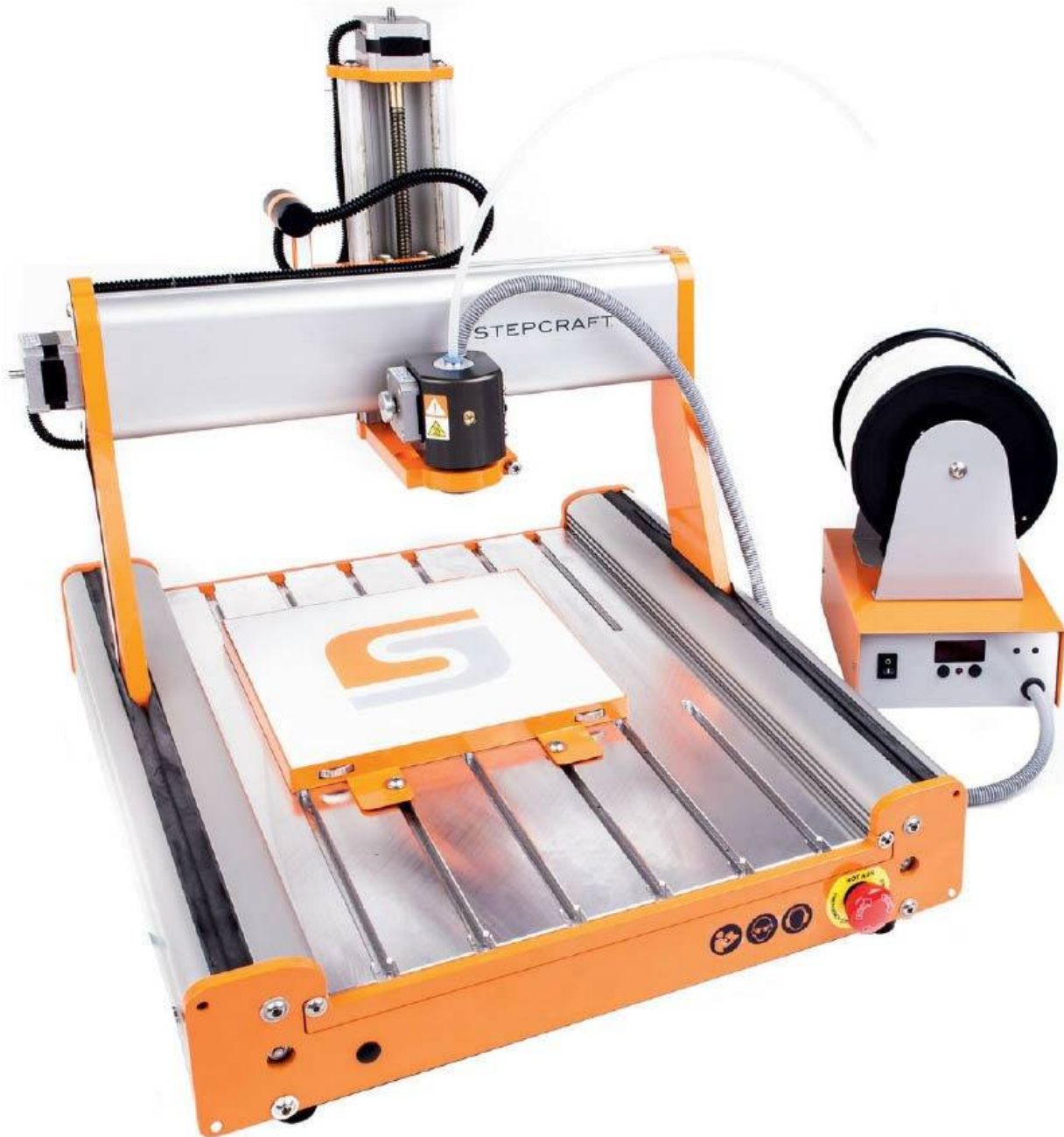
Fig. 1.21 A milling machine adapted for 3D printing
