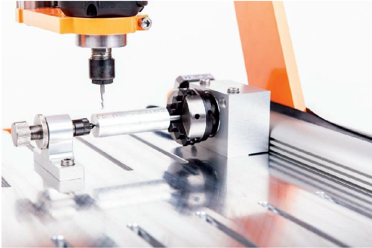
Fig. 1.22 A 4-axis upgrade with a tailstock (on the left)
