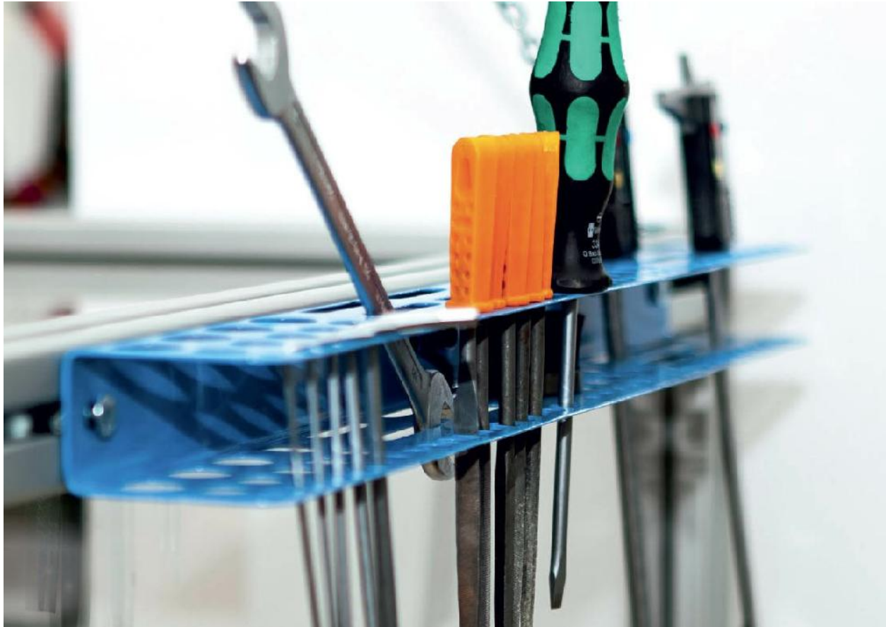
Fig. 5.4 An add-on tool holder
