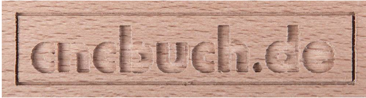
Fig. 4.14 Our first attempt at milling solid beech
