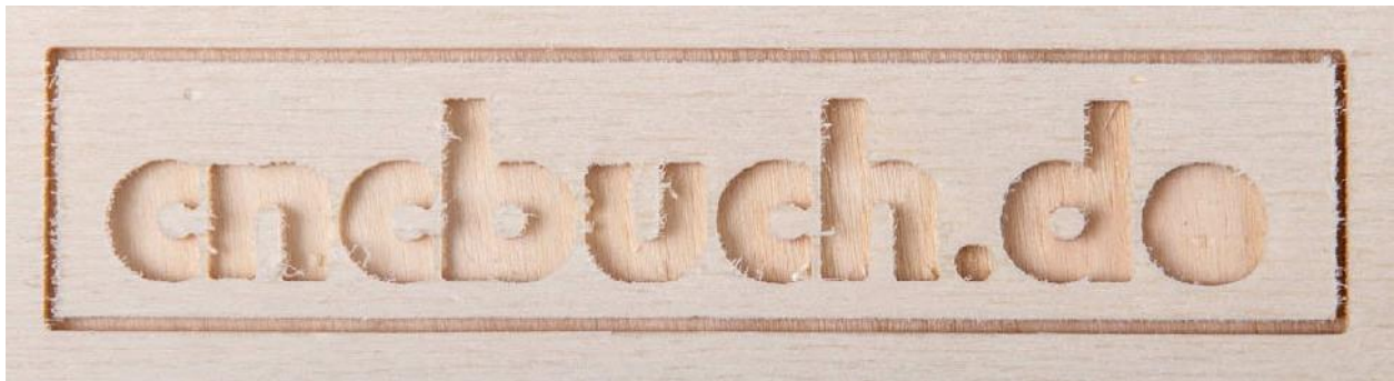
Fig. 4.8 A poor result produced using poplar plywood
