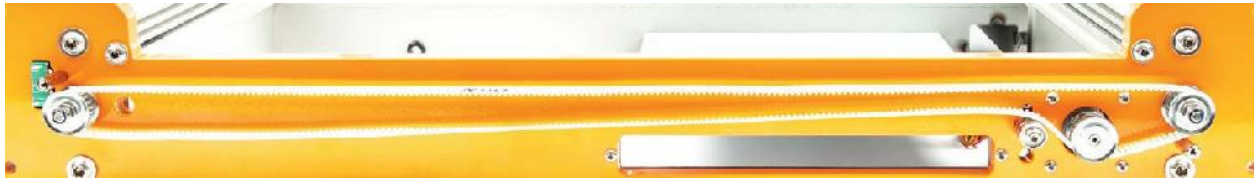
Fig. 2.75 The correctly mounted drive belt
