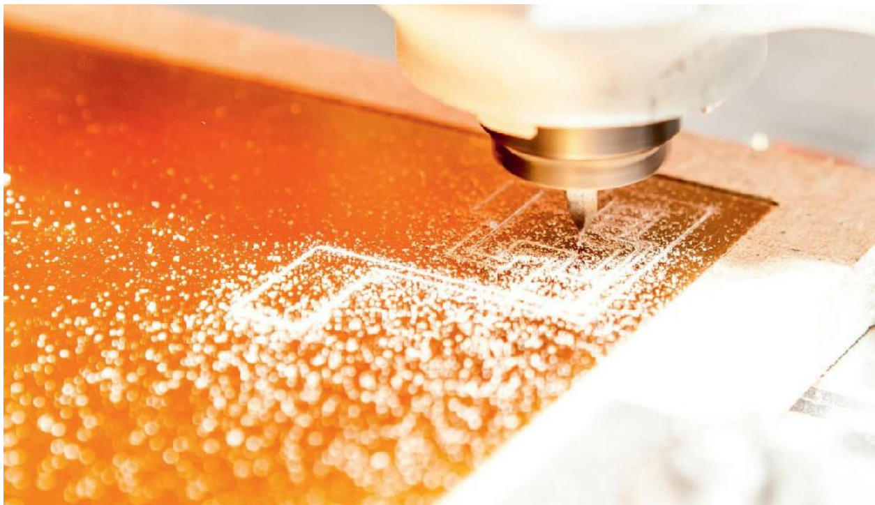
Fig. 1.15 Using isolation milling techniques to make a circuit board
