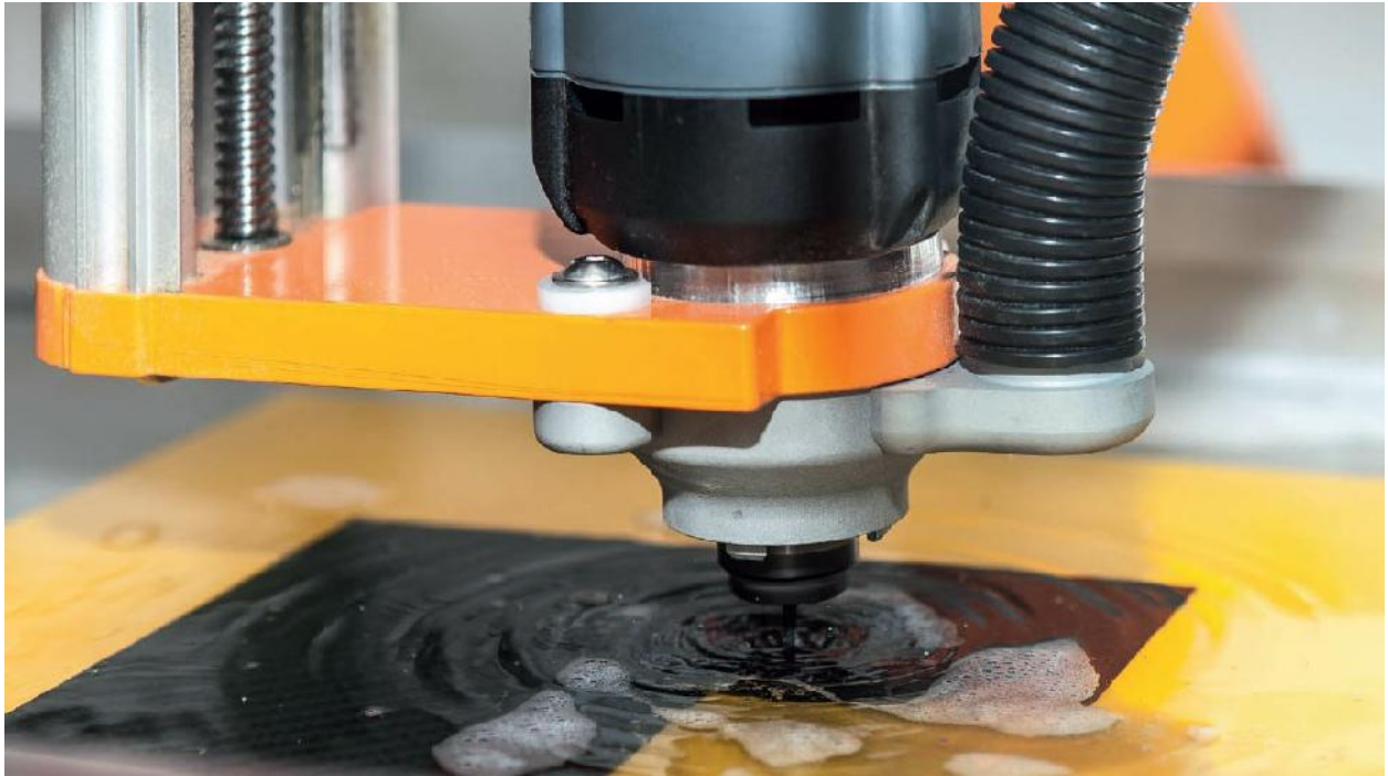
Fig. 6.18 Underwater milling in progress
