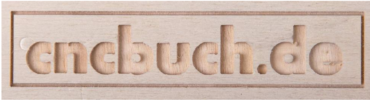
Fig. 4.12 The cleanest result so far using poplar plywood
