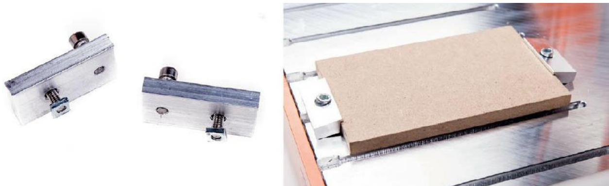
Fig. 1.18 Home-made clamps (left) and a clamping system for holding boards (right)
