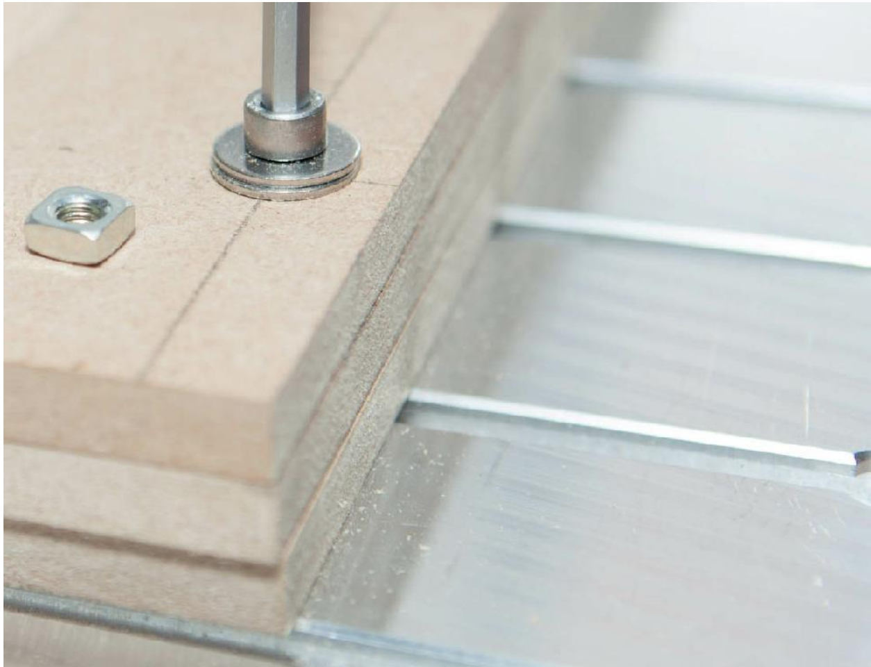
Fig. 6.35 Fixing multiple blanks to the machine table without using hold-down clamps
