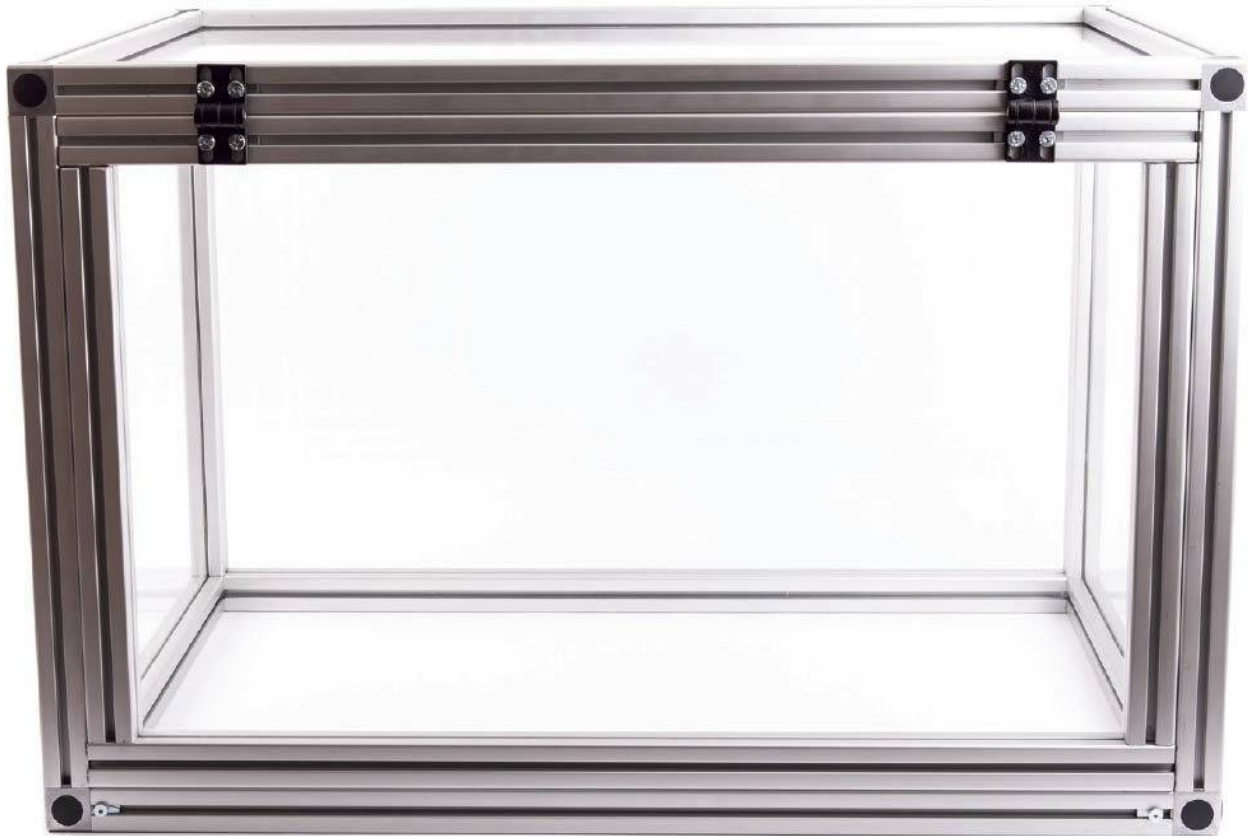
Fig. 5.2 The finished enclosure, showing the mounted Plexiglass sheets and the front hatch
