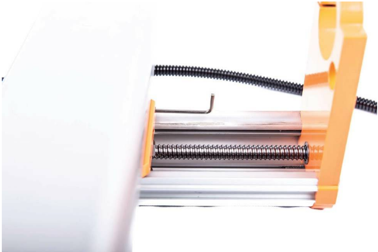
Fig. 2.46 Adjusting play in the X axis
