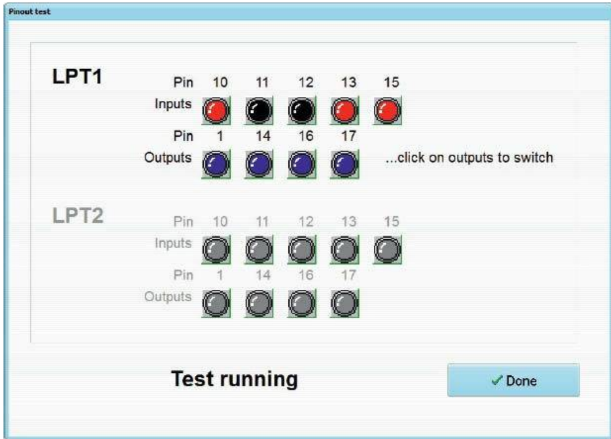
Fig. 5.25 The result of triggering the connected tool length sensor
