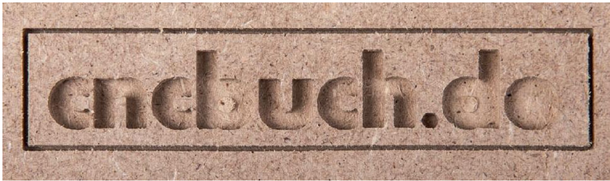
Fig. 4.6 The result of milling our pattern in MDF
