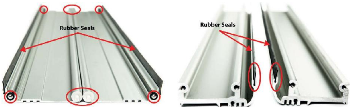
Fig. 2.65 Preparing the Y rails and the side panels of the Y axis
