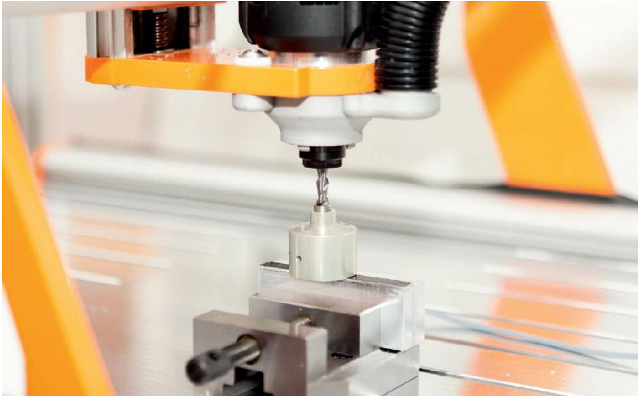
Fig. 5.28 Using a tool length sensor to determine the Z zero point
