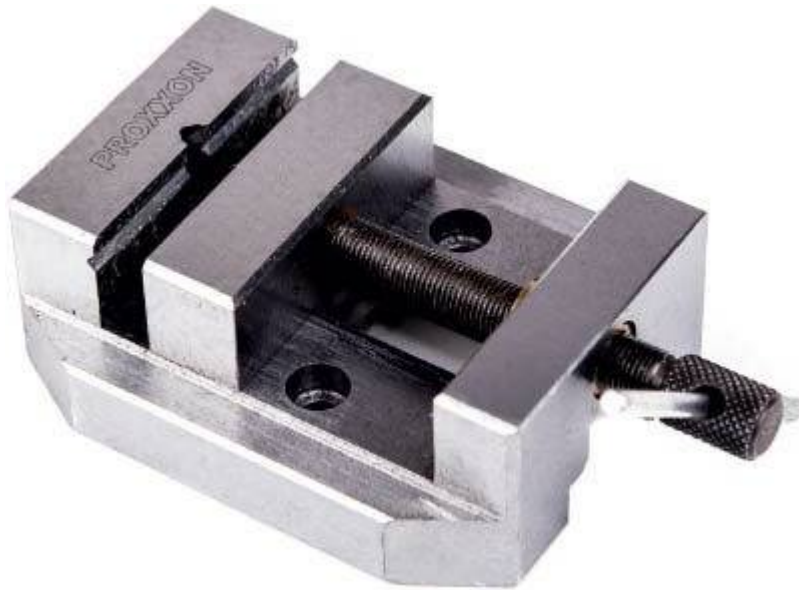
Fig. 1.17 A machine vise with centering grooves for holding rounded workpieces
