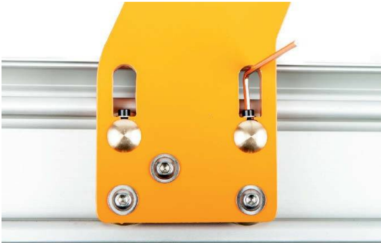
Fig. 2.36 Adjusting the play in the right-hand gantry rollers
