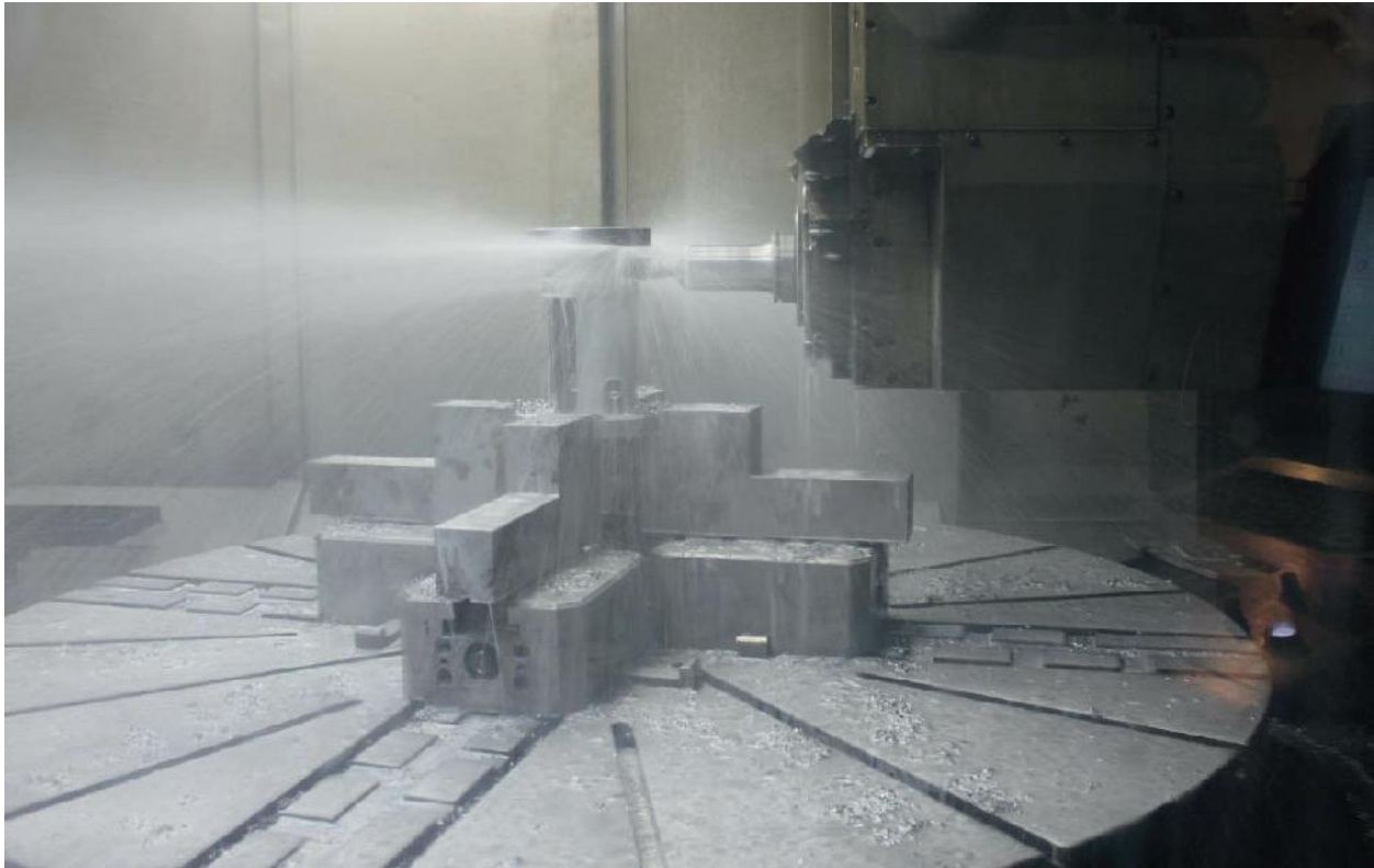
Fig. 1.3 An industrial CNC machine with a rotary machine table (the 4th axis)
