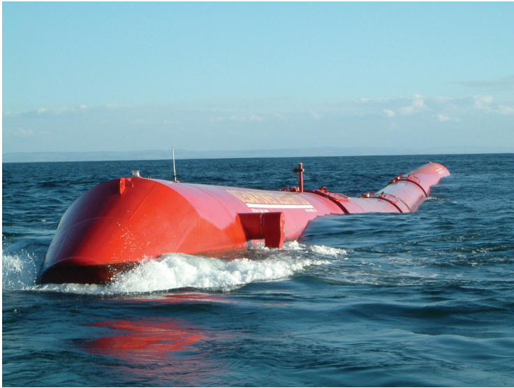
FIGURE 4.72 Pelamis WEC device at sea (Ocean Power Delivery Ltd). (Courtesy of R. Henderson, Renewable Energy , 31 (2), 271–283, 2006.)
