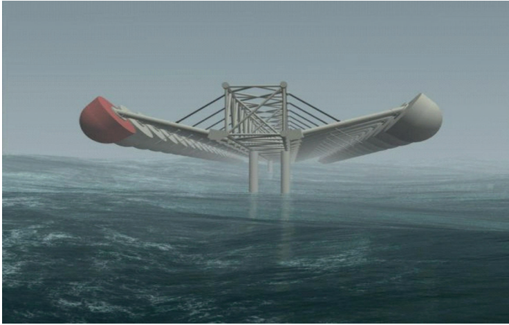
FIGURE 4.82 WSE position in storm protection mode. (Courtesy of M. Kramer, “The wave energy converter: Wave Star, a multi point absorber system,” Technical Report, Aalborg University and Wave Star Energy, Bremerhaven, Denmark.)
