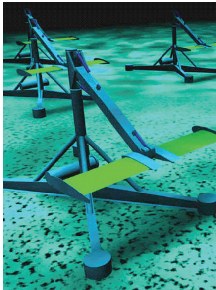
FIGURE 3.50 Stingrays mounted on the seabed. (Courtesy of Engineering Business Ltd., UK, “Stingray tidal stream generator,” available at: http://www.engb.com , March 2008.)
