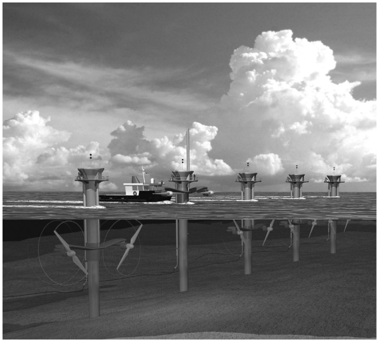
FIGURE 3.43 (See color insert following page 80.) SeaGen turbine farm. (Courtesy of Seaflow and SeaGen Turbines, Marine Current Turbines Ltd., available at: http://www.marineturbines.com , March 2008.)
