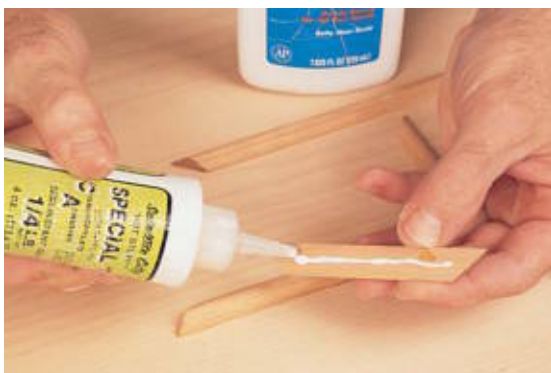
When applying moldings to flat work, spread a bead of white glue; then squeeze drops of CA along the glueline.
