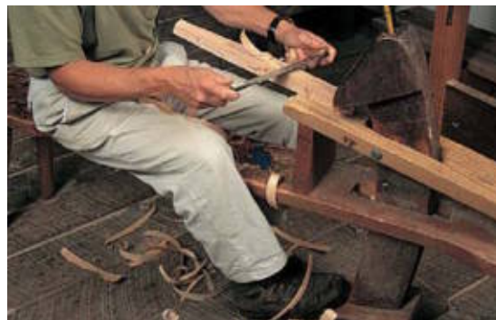
A shaving horse provides a quick way to hold the squares as you work them. Firm foot pressure tightens the head on the workpiece.
