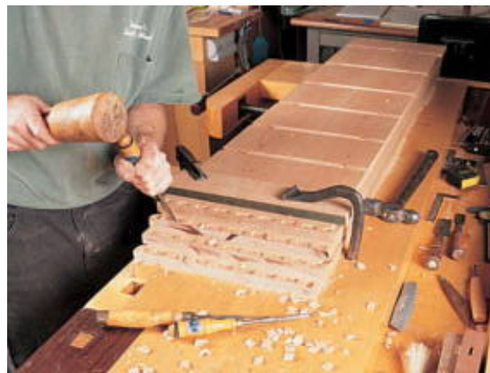
A holdfast uses a wedging action through the benchtop to keep a piece in position for handwork, especially for carving or chopping tasks.
