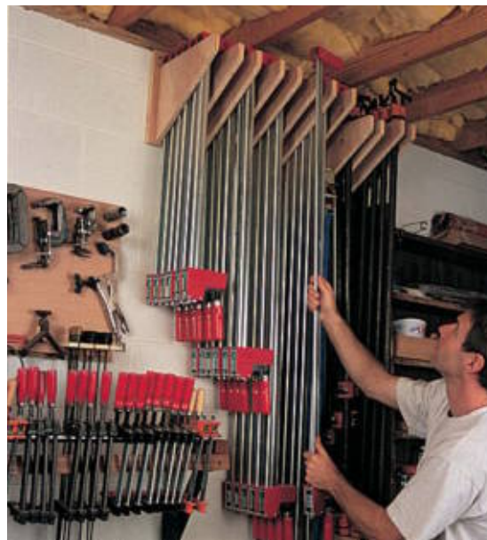
A set of plywood wall brackets organizes your bar clamps, making them readily accessible.
