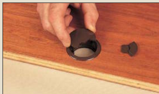
Tap the barbed grommet into the hole. A plastic cap reduces the opening for smaller runs of wire.
