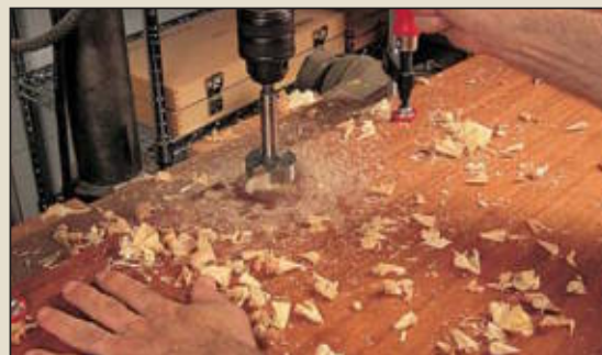
Use a Forstner bit to drill a hole equal to the ring diameter of the grommet.
