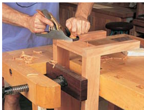
The open jaws of a shoulder vise allow larger workpieces to pass right through for easy clamping. The vise has a swiveling jaw to provide even pressure onto tapered workpieces.
