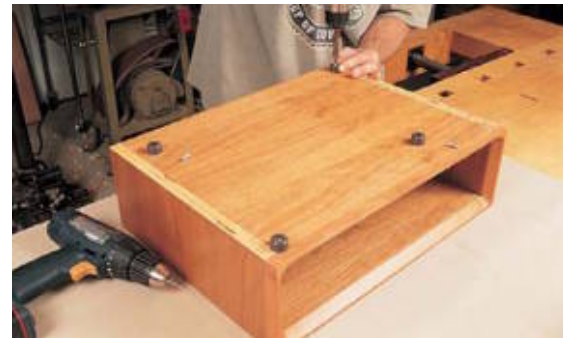
Blocks installed on the outside corners are a simple way to elevate a small case.
