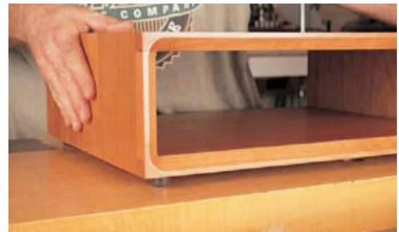
When the case is turned right side up, a slight rise creates an attractive shadow line.
