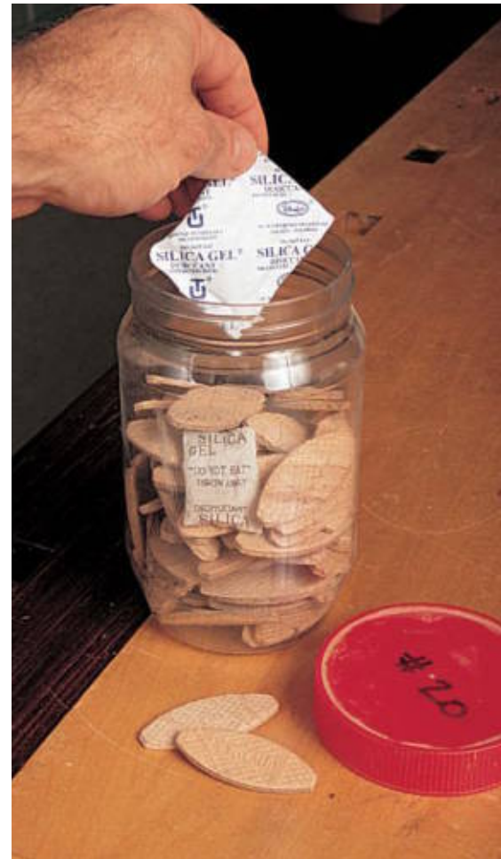
Drop a bag or two of desiccant into a jar filled with plate biscuits to keep them dry.
