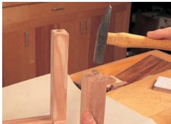
Small plastic furniture glides are simply nailed in place.
