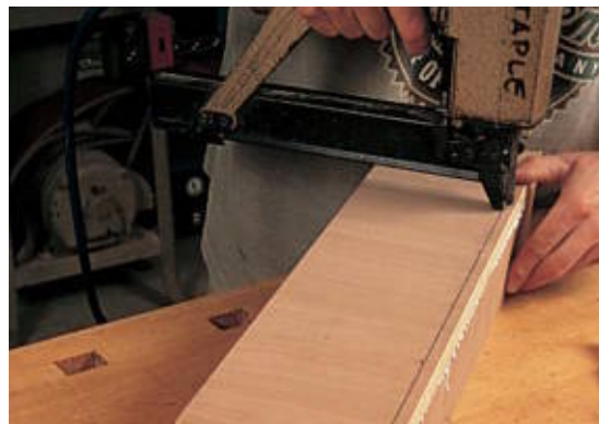
A simple L-shaped foot can be used for extra support under a base cabinet.
