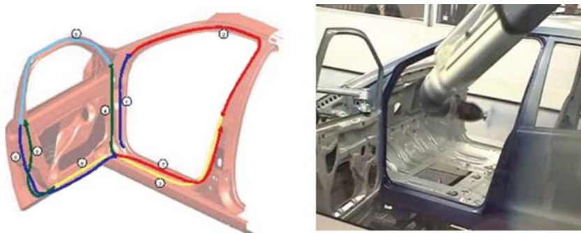
Fig. 8.38 Spray pattern of interior applications with electrostatic high-speed rotation.
