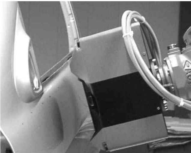
Fig. 8.31 Robot-guided, contactless online measurement of color and surface leveling (source: Optronic).
