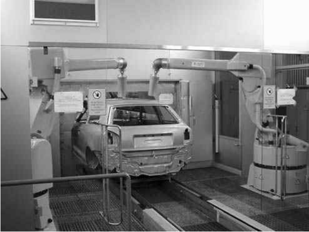
Fig. 8.30 Robot-guided contactless online measurement of film thickness.
