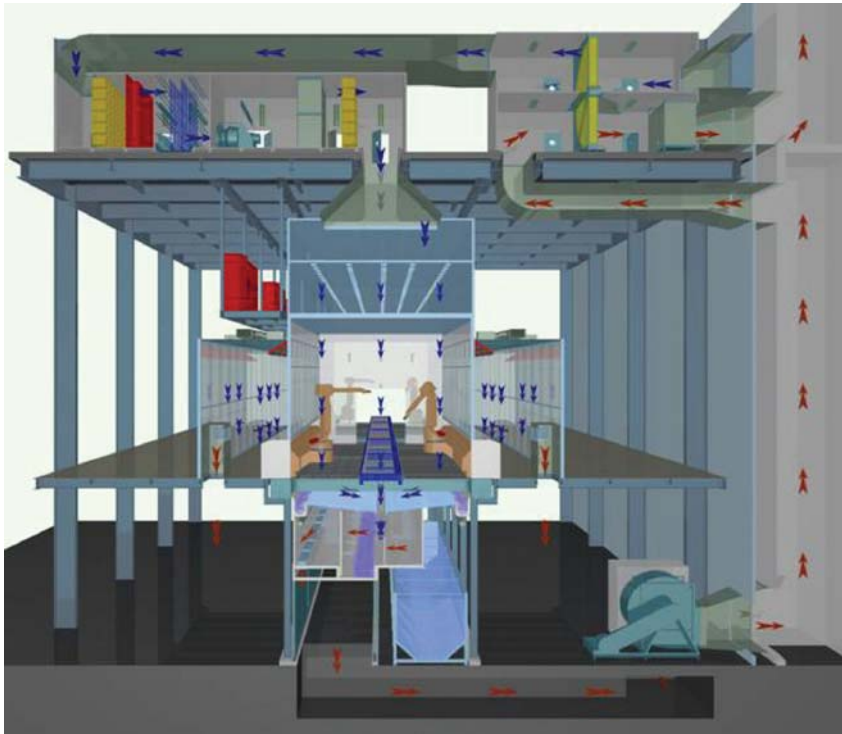
Fig. 8.8 Cross section of a spray booth.
