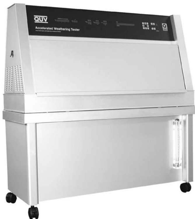
Fig. 12.48 Exterior view of a typical QUV tester.
