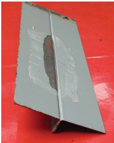
Fig. 12.57 Typical test panel for contact corrosion and sealer testing after 10-week climate change test (left panel: Steel).
