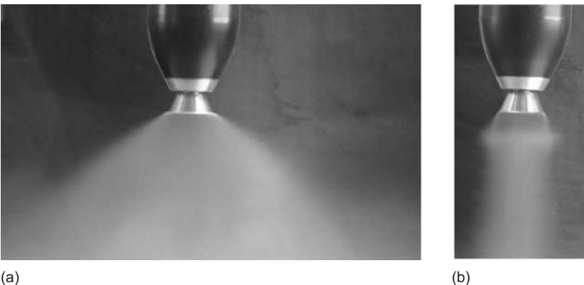
Fig. 8.37 Spray pattern settings for widths between 50 (b) and 600 mm (a).
