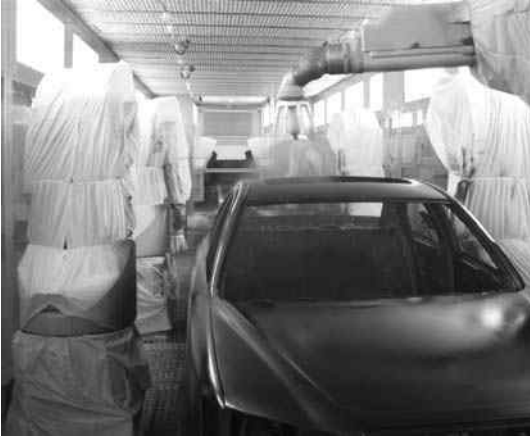
Fig. 8.36 Second application step of metallic base coats with high-speed-rotating atomizer and electrostatic paint charging.
