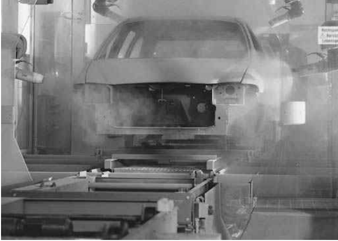
Fig. 5.27 Powder primer surfacer application with corona powder guns on a car body (source: BASF coatings).
