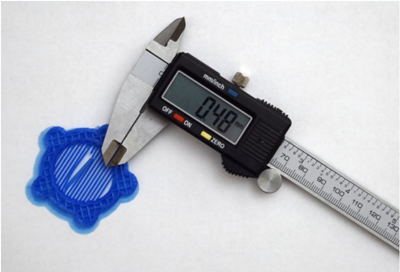
Figure 4-17. Calipers show an extrusion width of .48mm extruded from a .4mm nozzle
