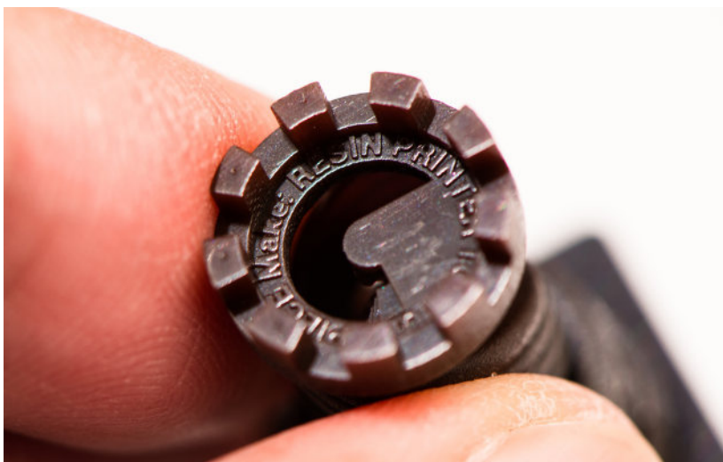
Figure 5-9. Make: magazine's twisted-rook “torture” test, used to push the capabilities of resin printers, printed here with the Kudo3D
