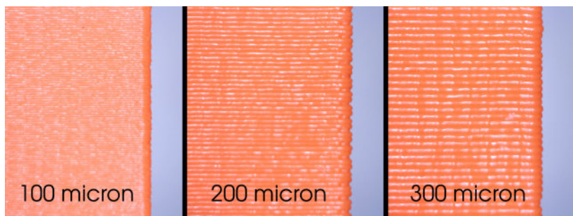
Figure 4-2. A close-up image of three layer heights printed at (left to right) 100 microns, 200 microns, and 300 microns
