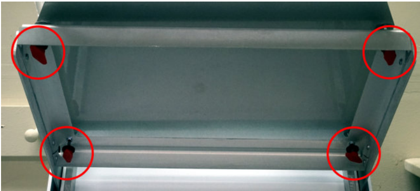
Figure 4-28. A view from underneath the Type A Machines Series 1 printer, showing the four bed-leveling screws with 3D printed handles
