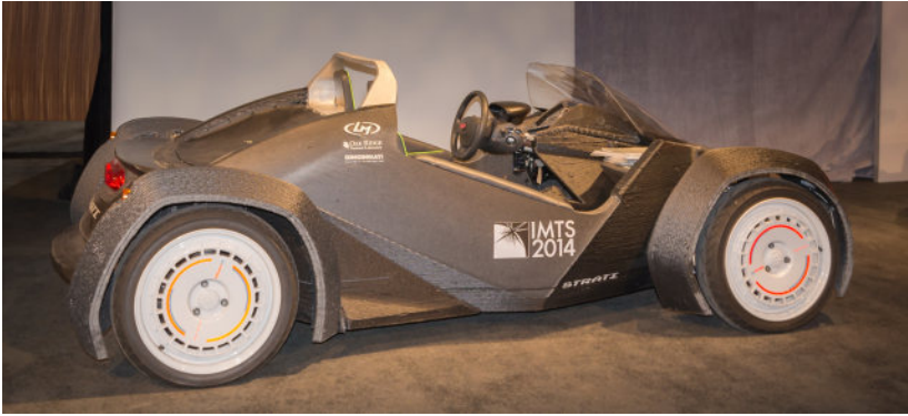
Figure 3-1. Detroit, January 2012, Local Motors Strati, a 3D printed concept car using rapid prototyping (Steve Lagreca, Shutterstock.com)
