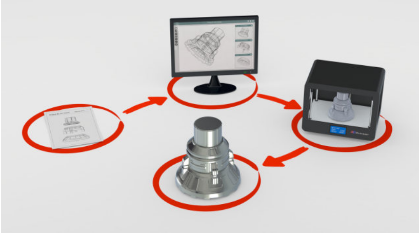
Figure 7-4. The workflow from idea to finished 3D print going clockwise from the left: 2D drawing, CAD file generation, 3D printed prototype, final piece
