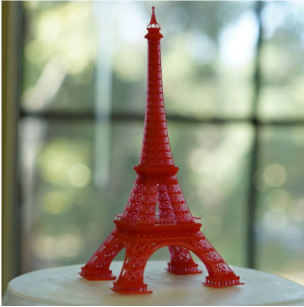
Figure 5-2. Eiffel Tower model printed on an SLA printer (3D model credit: Pranav Panchal)
