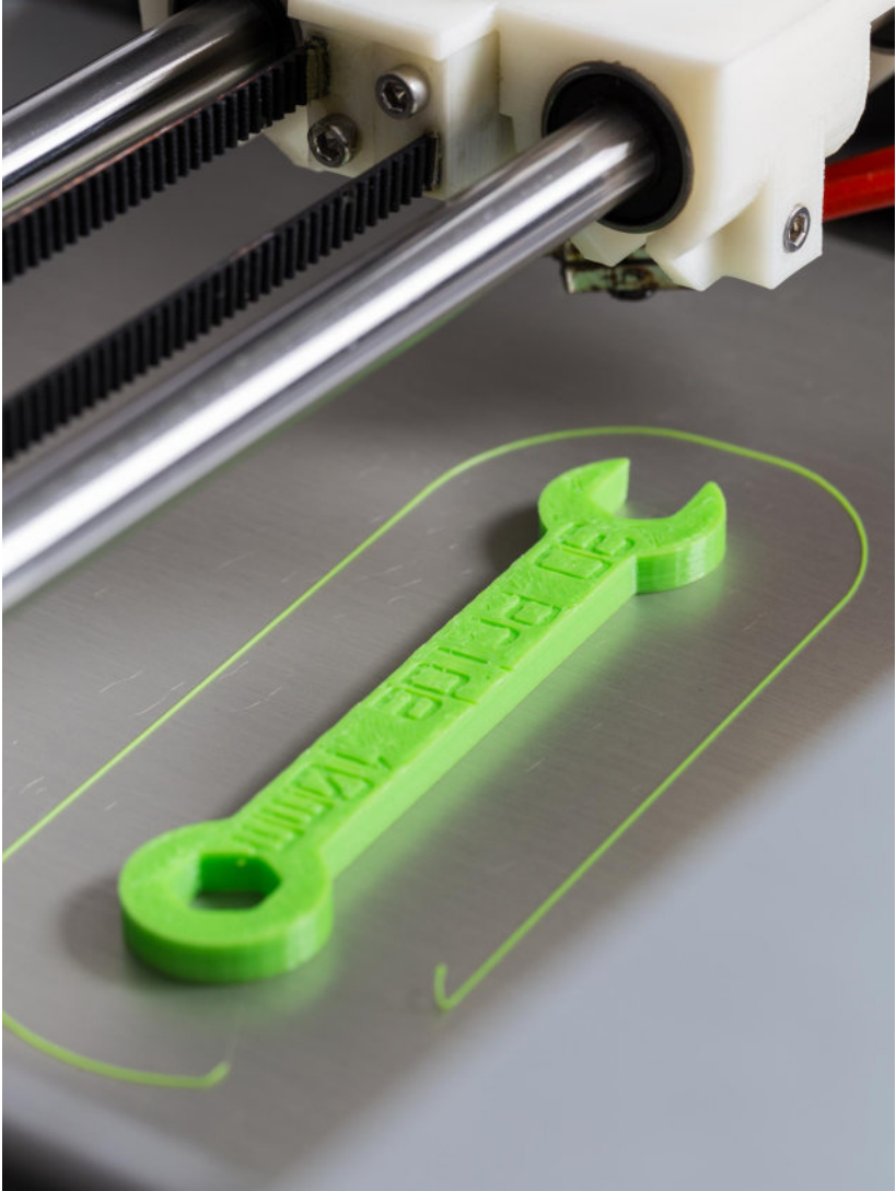
Figure 13-2. In the future, a tool manufacturer will let you download the CAD file and 3D print it at home or at your local hardware store
