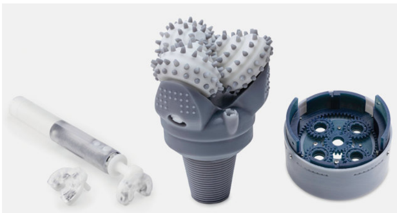
Figure 5-12. Sample prints from a FormLabs Form 2 printer. These objects were printed separately and then hand-assembled.
