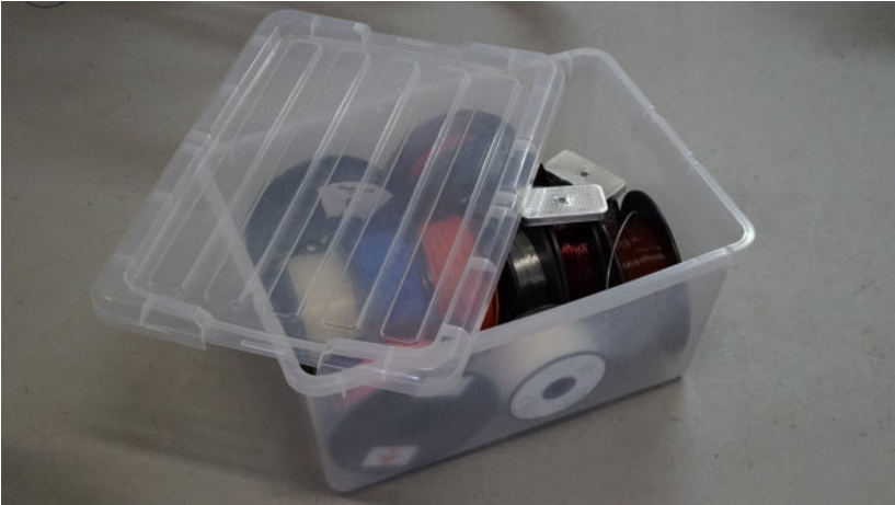
Figure 4-20. Spools of filament stored in a mostly airtight container, with desiccant pouches added
