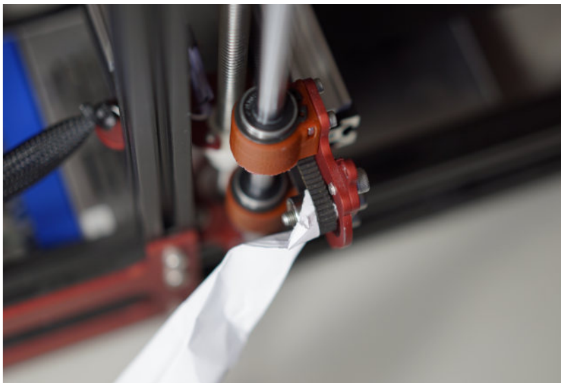
Figure 12-6. 3D printer belt and pulley crushing paper, showing the potential pinch hazards
