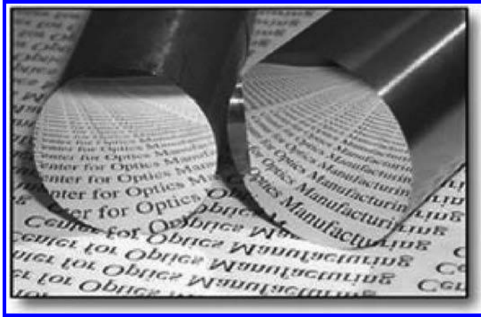
FIGURE 1.5 Molds with diamond turning (center for optic manufacturing).
