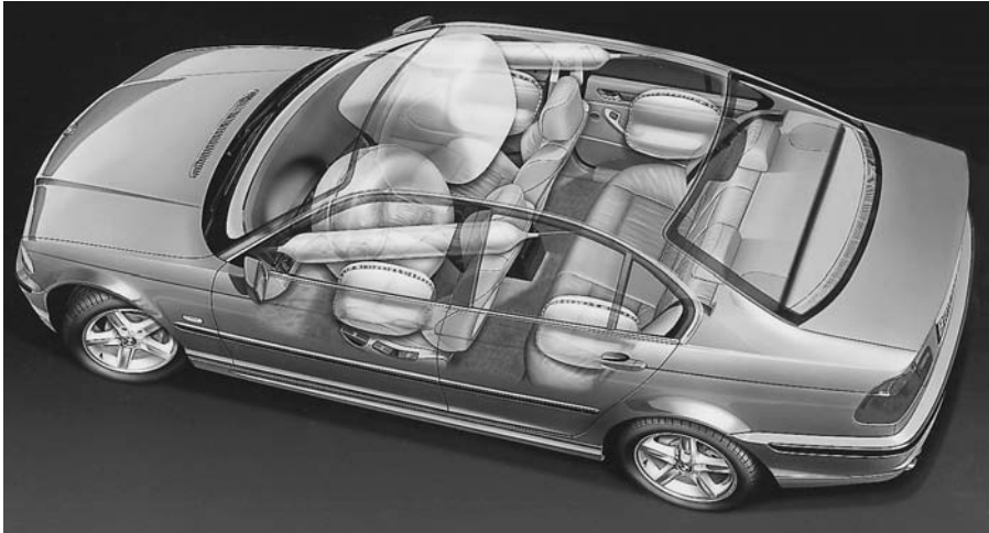
Fig. 4.25 BMW passenger car with air bags for the front, sides and head (front and back).
