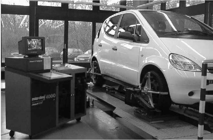
Fig. 3.162 Computer-aided wheel kinematics measuring device of the Chassis/Simulation Technology Laboratory of the University of Applied Science, Cologne. Changes in the position of the wheels in the course of body lifting and lowering movements can also be measured by means of actuators which are integrated into the test stand.
