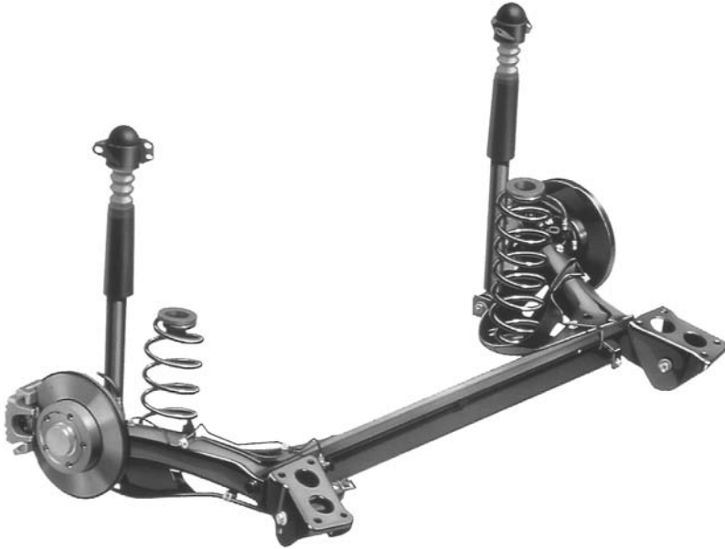
Fig. 1.30 Twist-beam suspension of the VW Golf IV (1997), VW Bora (1999) and Audi A3 (1996). The rubber-metal bearings of the axle body are set at 25^\circ to the transverse suspension of the vehicle in order to improve the self-steering properties of the suspension together with the rigidity of the bearings which varies in three directions in space. Compared with the previous model, it was possible to reduce unwanted lateral-force toe-out steer resulting from link deformation by 30% to approximately 1 mm per 500 N of lateral force. Figure 1.72 shows the four-wheel drive version of the VW Golf IV.
