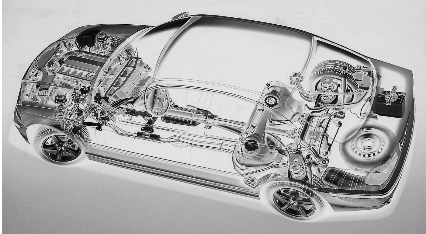
Fig. 1.32 Front-mounted engine, rear-mounted drive (BMW 3 series E46, 1998). The manual transmission is flange-mounted on the engine, which is longitudinally positioned over the front axle. The rear-axle differential is driven by means of a propshaft. The fuel tank is situated in front of the rear axle for safety in case of an accident. The battery was placed in the boot in order to achieve a balanced 50:50 axle-load distribution. Figure 1.1 shows the rear axle in detail.
