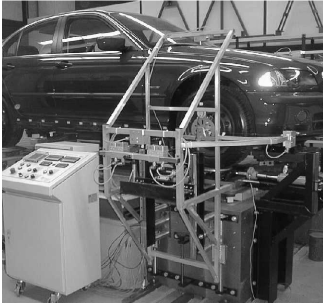
Fig. 3.163 Elastokinematics test stand of the Chassis/Simulation Technology Laboratory of the University of Applied Science, Cologne. The movements of the wheels are measured by a combined system of filament potentiometers and inclinometers constructed on the basis of a system of error and fault minimization; forces are measured by means of force transducers. A computer system is used for measurement, stipulation of the required values and evaluation. Forces can be applied with the normal tyres left in place or via wheel replacement carriers; air-sprung sliding plates are used to minimize friction.
