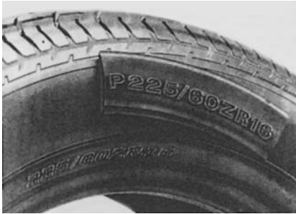
Fig. 2.17 ZR tyres manufactured specially for the American market and marked with a 'P' do not meet the European standard and are therefore not authorized here (photograph: Dunlop factory).
