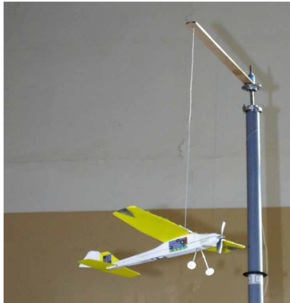
Figure 28. Models of an electric airplane powered by a resonant single-conductor system
