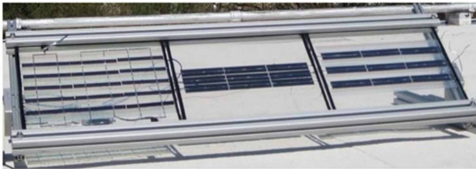
Figure 18. Experimental setup for the measurement of the cell temperature of the holographic panels. The coupons had the following arrangement (Left) 2 to 1 holographic coupon, (Middle) packed reference coupon, (Right) 1 to 1 holographic coupon. The system was pointed south and tilted for latitude.
