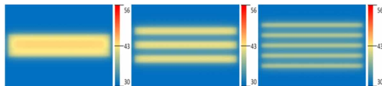
Figure 22. Model derived heat maps at the solar cell layer for an EPV of 800 \text{ Wm}^{-2} and a heat transfer of 30 \text{ Wm}^{-2} for the glass surfaces for the test coupon configurations. The color scales varies from 30C (light blue) to 56C (bright red).
