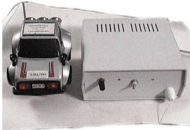
Figure 12. Model of a mobile mechanism with a single-conductor power supply system
