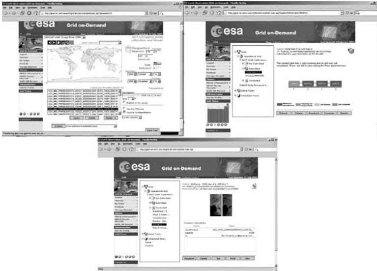
Figure 11.7 The ASAR G-POD environment. The user browses for and selects products of interest (upper left panel). The system automatically identifies the subtasks required by the application and distributes them to the different computing elements in the grid (upper right panel). Results are presented to the user (lower panel).
