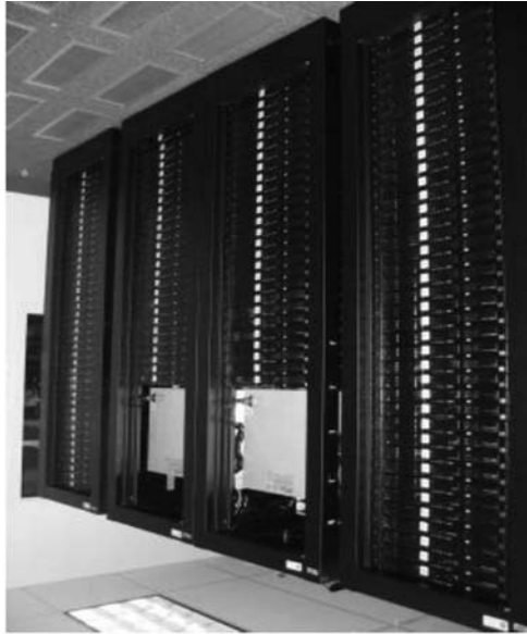
Figure 2.2 Thunderhead Beowulf cluster (512 processors) at NASA's Goddard Space Flight Center in Maryland.
