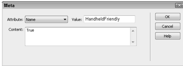
Figure 3-8: The Handheld-Friendly meta tag tells search engines and others that this page displays well on mobile devices.
