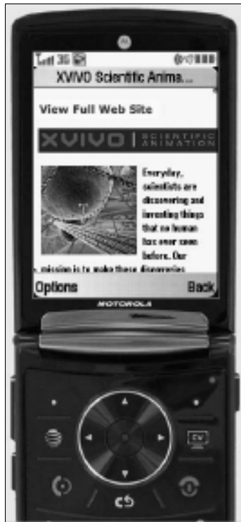
Figure 3-3: This mobile version of the XVIVO Web site was created with simple XHTML MP code so it displays well even in the limited browser on the Motorola RAZR.
