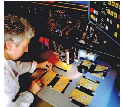
Troubleshooting an electronic circuit board.
