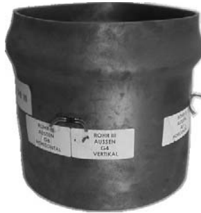
Fig. 10. Axially loaded pipe with L/D=1 after testing.
