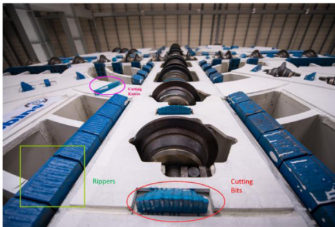
Figure 4.52 Terra Invader rig used for deep drilling. Courtesy of Herrenknecht AG.
