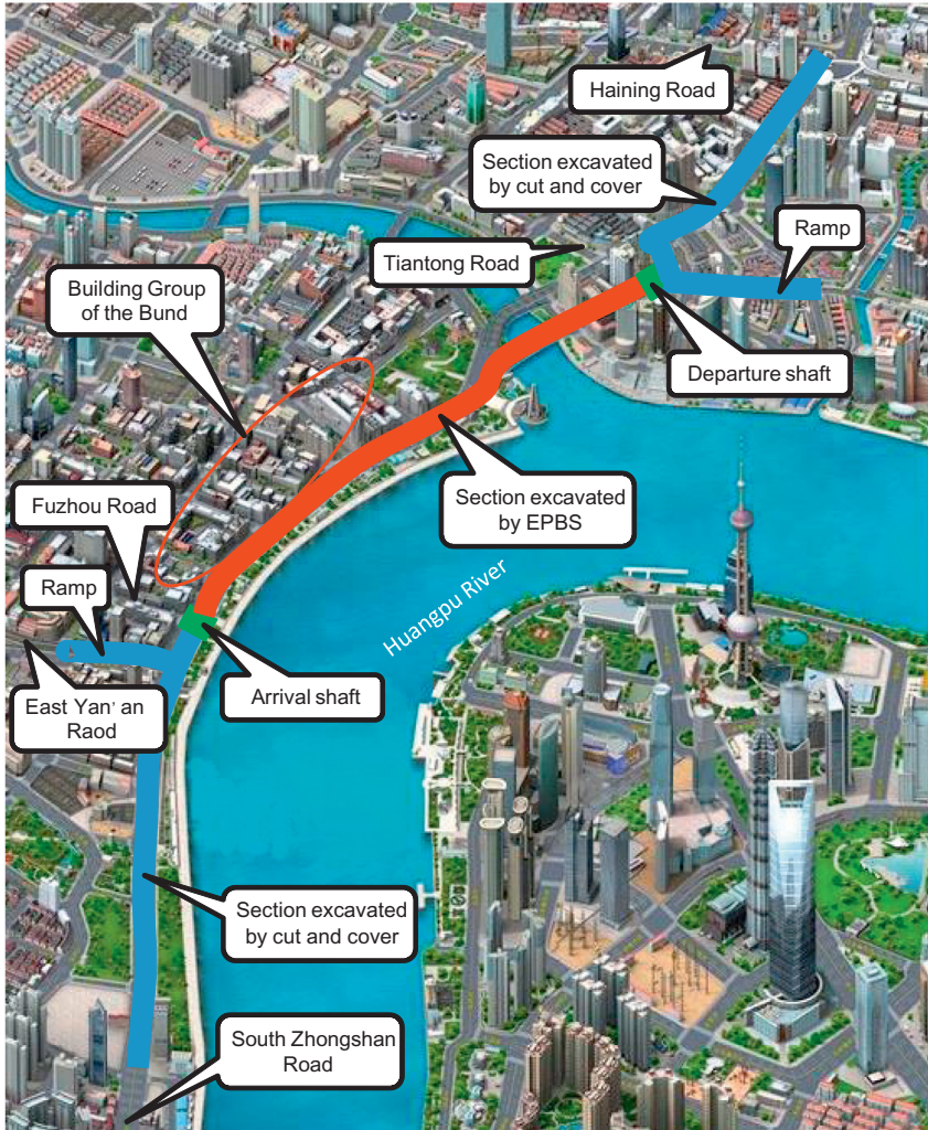
Figure 4.79 General layout of the Bund Tunnel.
