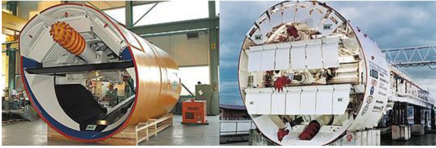
Figure 4.48 Two kinds of partial-face excavation machines. Courtesy of Herrenknecht AG.
