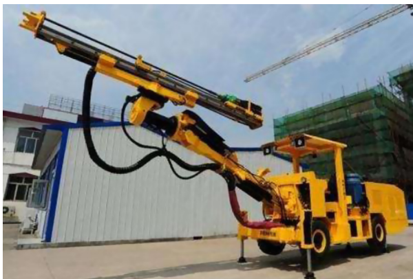
Figure 4.28 A tunnel jumbo drilling rig.
