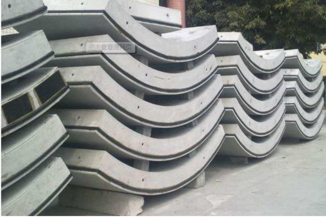
Figure 4.57 Stacked precast segments.
