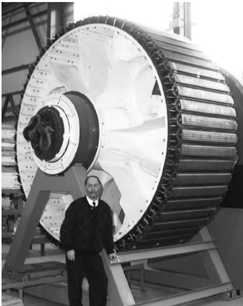
FIGURE 15.7 Rotor, TWT multipole synchronous generator. (Courtesy M.Torres Group, Navarra, Spain.)
