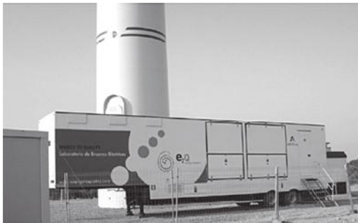
FIGURE 15.22 Experimental assays: voltage dip generator and TWT.
