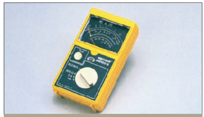
FIGURE 9-25 Battery-operated MEGGER ® . Courtesy of Biddle Instruments.
