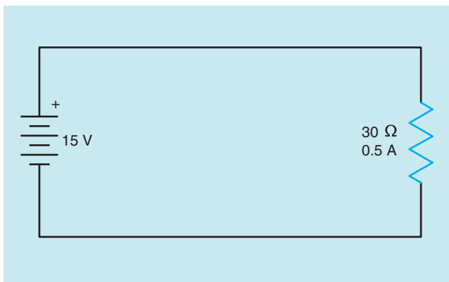
FIGURE 4-1 Resistor used to limit the flow of current.
