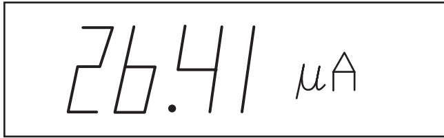
FIGURE 8-36 Display indicates a current of 26.41 microamperes.
