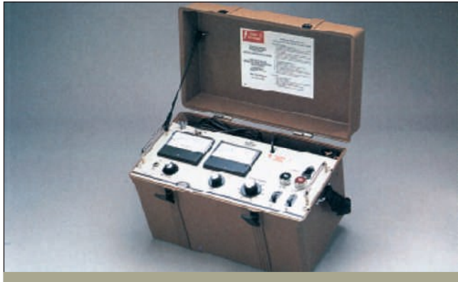
FIGURE 15-31 A dielectric test set. Courtesy of Biddle Instruments.
