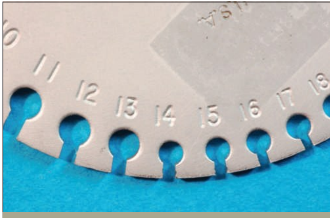
FIGURE 9-3 One side of the wire gauge is marked with the AWG size.
