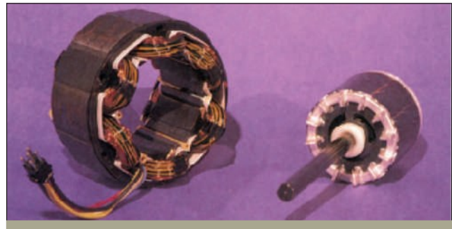
FIGURE 19-36 Stator winding and rotor of a shaded-pole induction motor. Courtesy of A. O. Smith.
