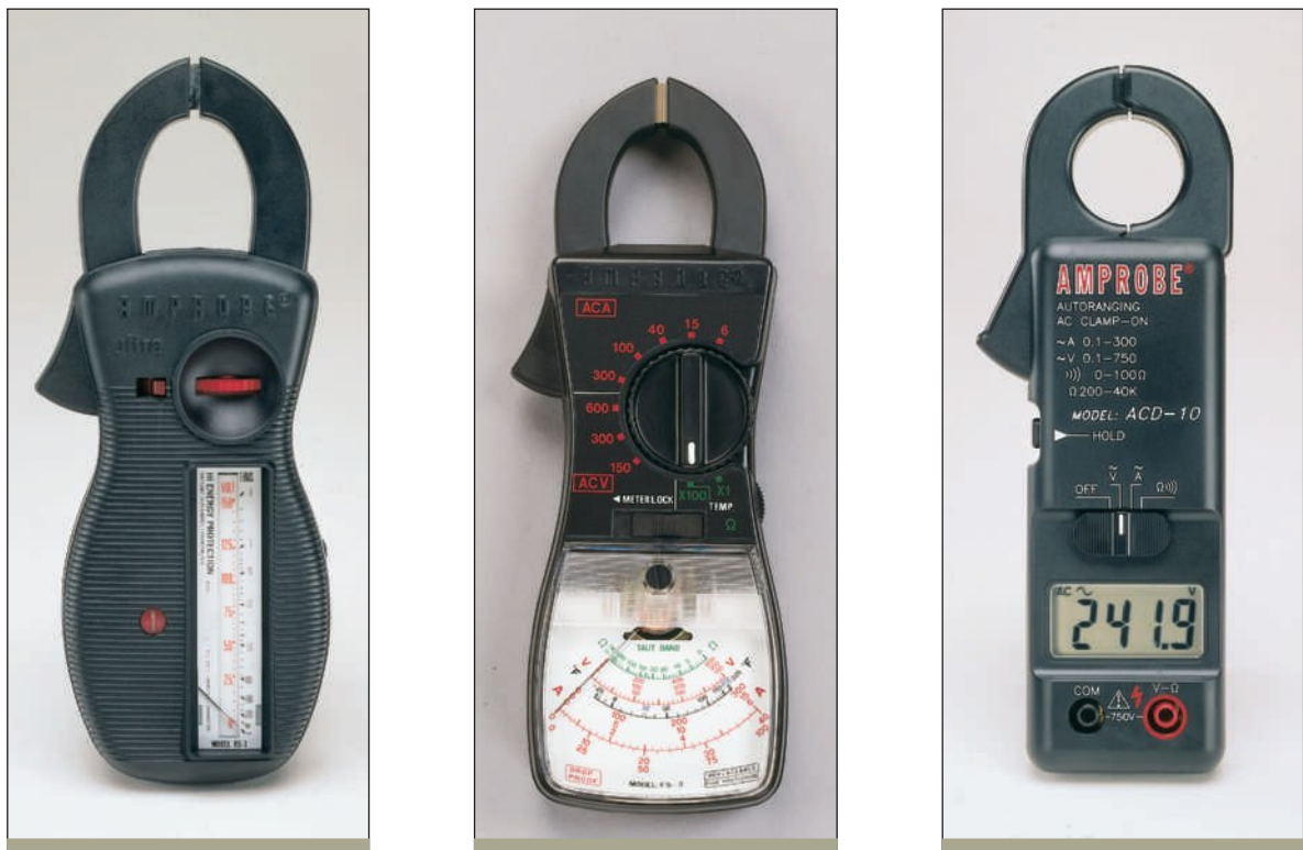
FIGURE 8-22 (A) Analog type clamp-on ammeter with vertical scale. (B) Analog type clamp-on ammeter with flat scale. (C) Clamp-on ammeter with digital scale. Courtesy of Amprobe Instrument.
